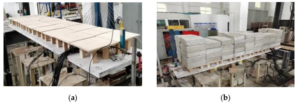
Figure 5. Test photos: (a) The upper floor of the board frame; (b) Live loading diagram.
