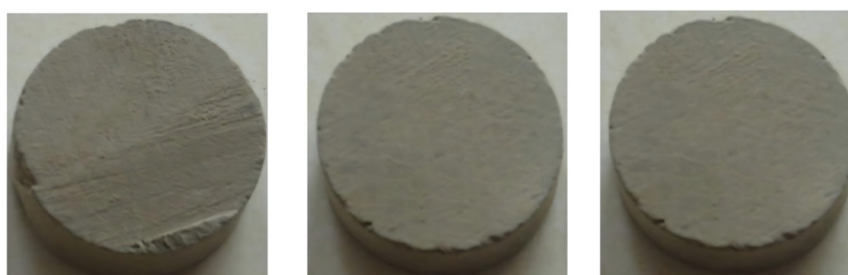
Figure 1. Typical deep oil reservoir mudstone samples.
