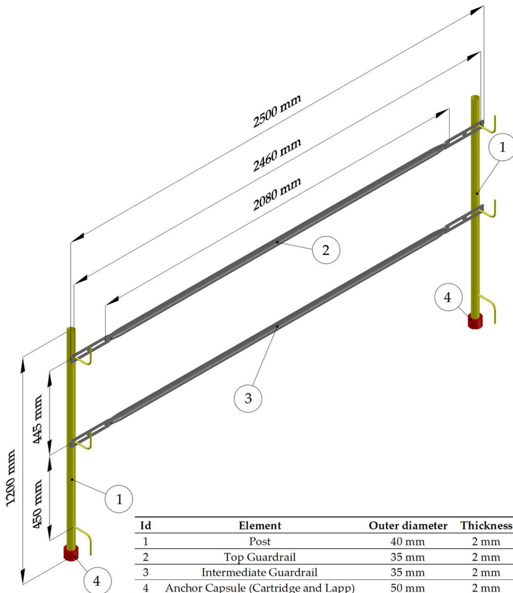
**Figure 4.** Description of the set of traditional elements (upright and horizontal railing) used as TEPS.
