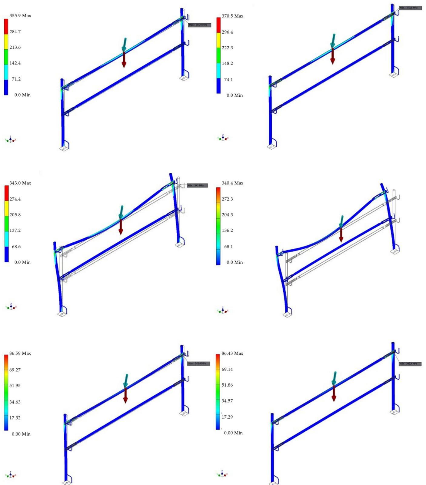
Figure A5. FEA von Mises stress in tests 7 and 8 for alternative materials: AL (top left), CI (top right), PET (centre left), PVC (centre right), GRFP (bottom left) and CRFP (bottom right).
