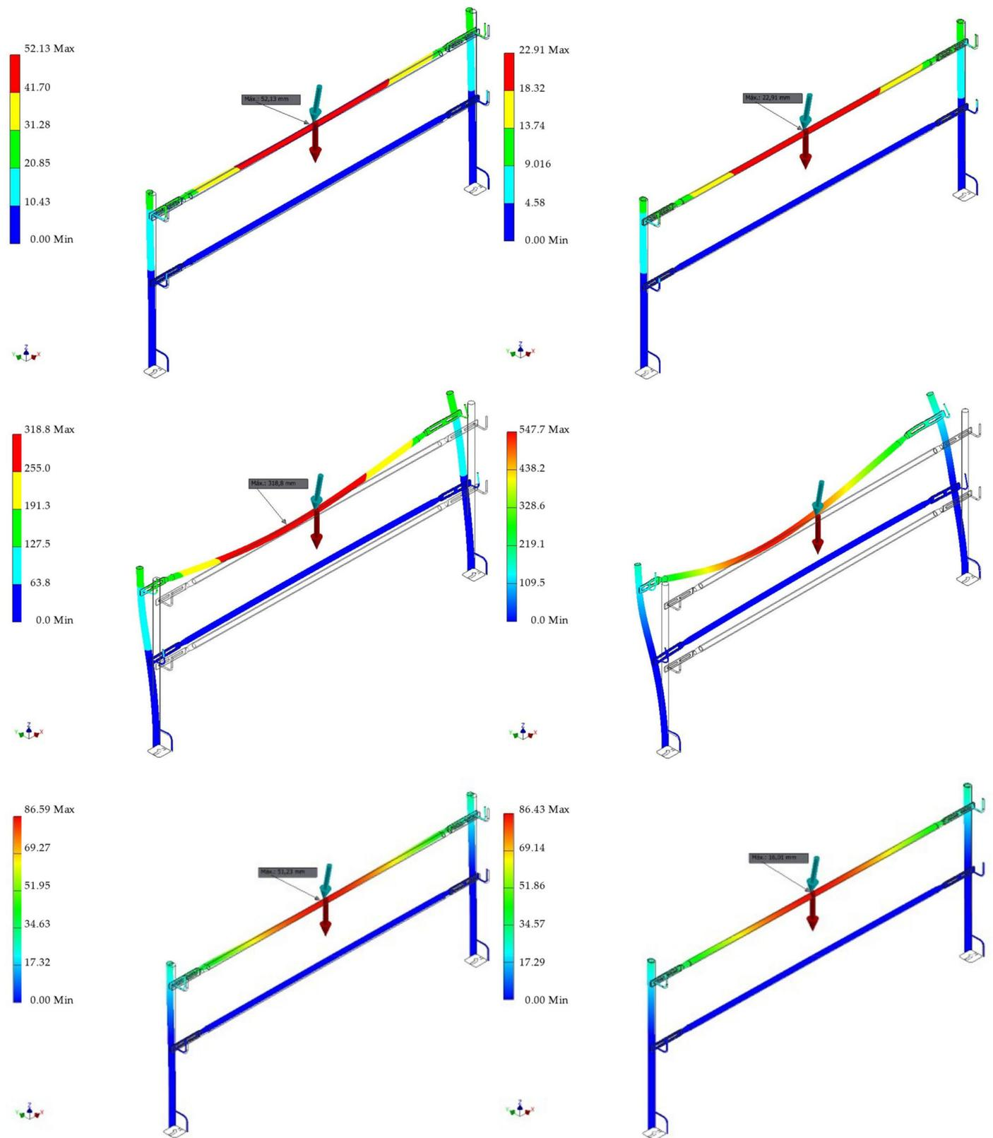
**Figure A4.** FEA deflection in test 6 for alternative materials: AL (top left), CI (top right), PET (centre left), PVC (centre right), GRFP (bottom left) and CRFP (bottom right).
