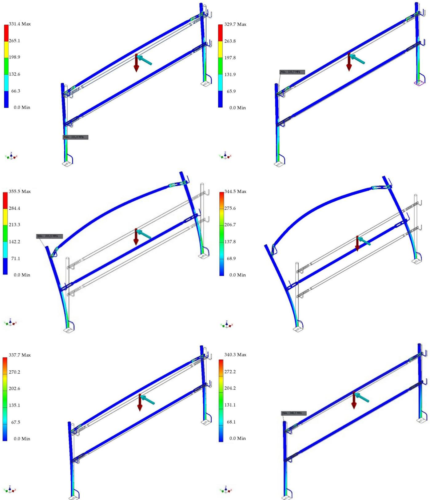
Figure A1. FEA deflection in test 1 for alternative materials: AL (top left), CI (top right), PET (centre left), PVC (centre right), GRFP (bottom left) and CRFP (bottom right).
