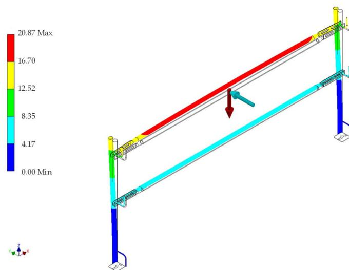
**Figure 6.** FEA deflection in test 1 for reference material (galvanised steel).
