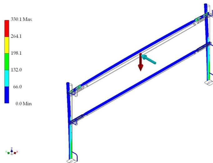
**Figure 7.** FEA von Mises stress in tests 2 and 3 for reference material (GS).
