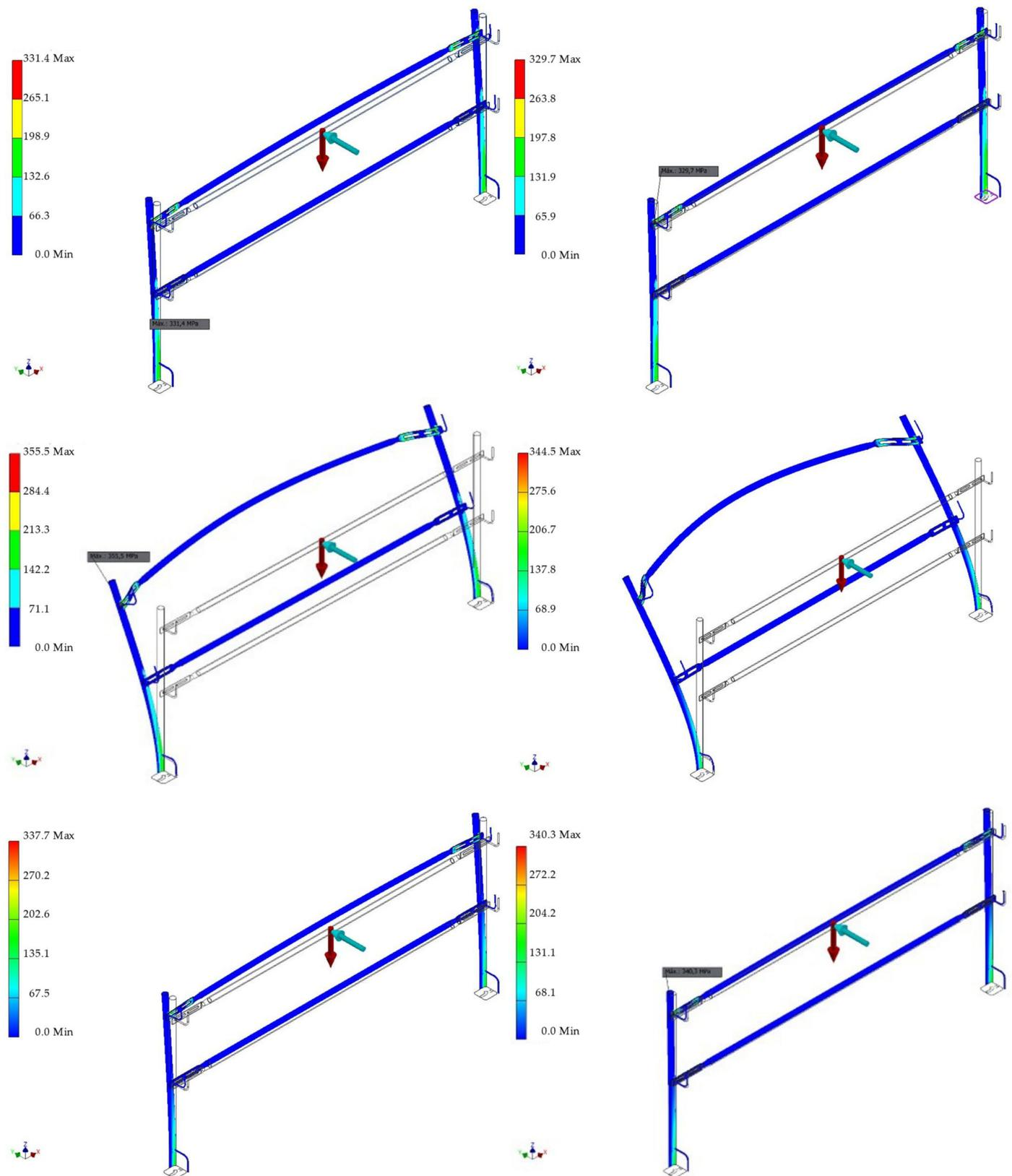
**Figure A2.** FEA von Mises stress in tests 2 and 3 for alternative materials: AL (top left), CI (top right), PET (centre left), PVC (centre right), GRFP (bottom left) and CRFP (bottom right).
