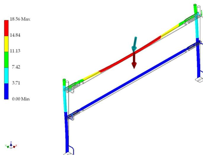
**Figure 9.** FEA deflection in test 6 for reference material (GS).
