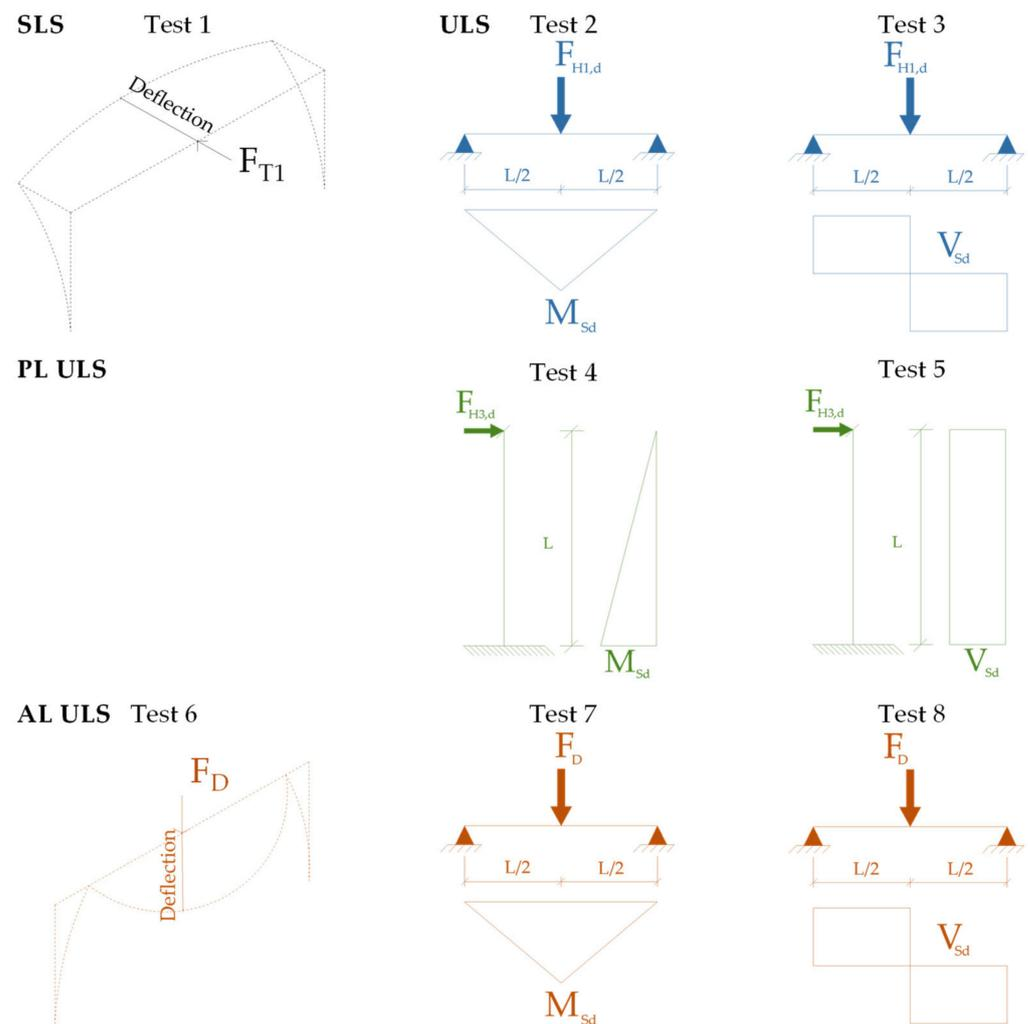
**Figure 5.** Diagrams of forces and moments of the tests carried out.
