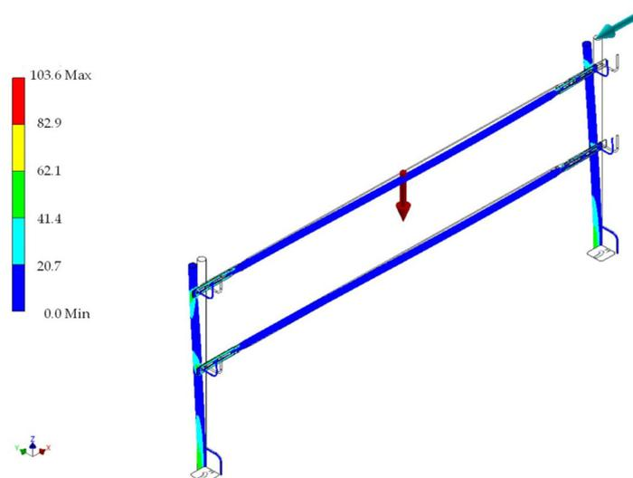
**Figure 8.** FEA von Mises stress in tests 4 and 5 for reference material (GS).
