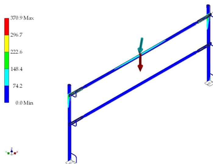
**Figure 10.** FEA von Mises stress in tests 7 and 8 for reference material (GS).
