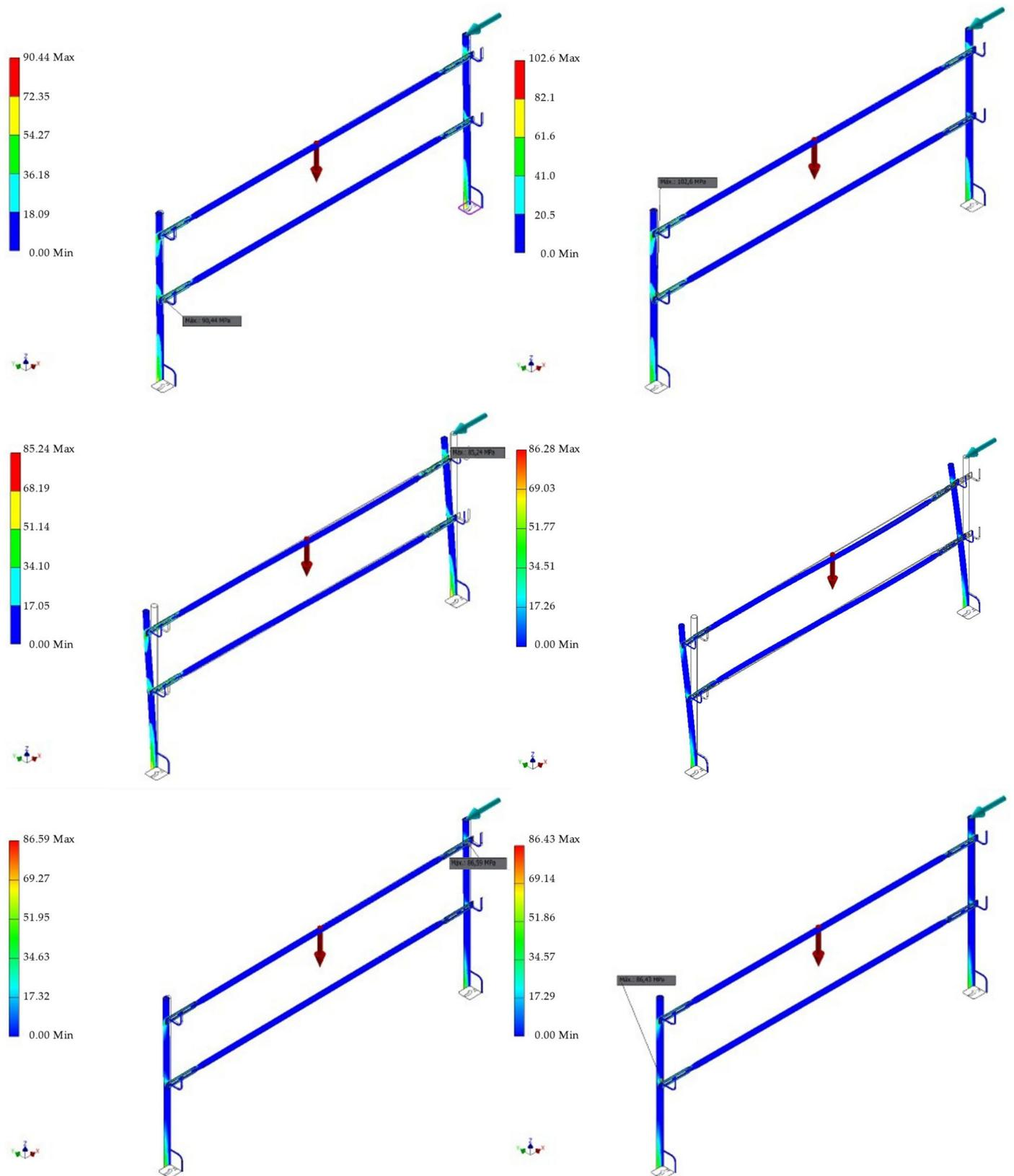
**Figure A3.** FEA von Mises stress in tests 4 and 5 for alternative materials: AL (top left), CI (top right), PET (centre left), PVC (centre right), GRFP (bottom left) and CRFP (bottom right).
