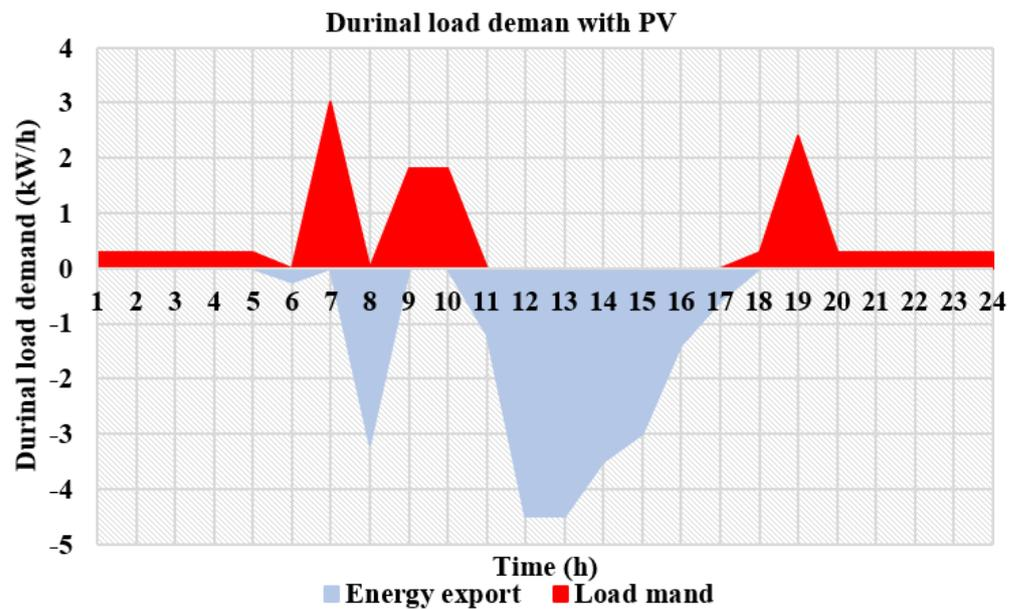
Figure 8. Load profile pattern per day of USLAs using PV.
