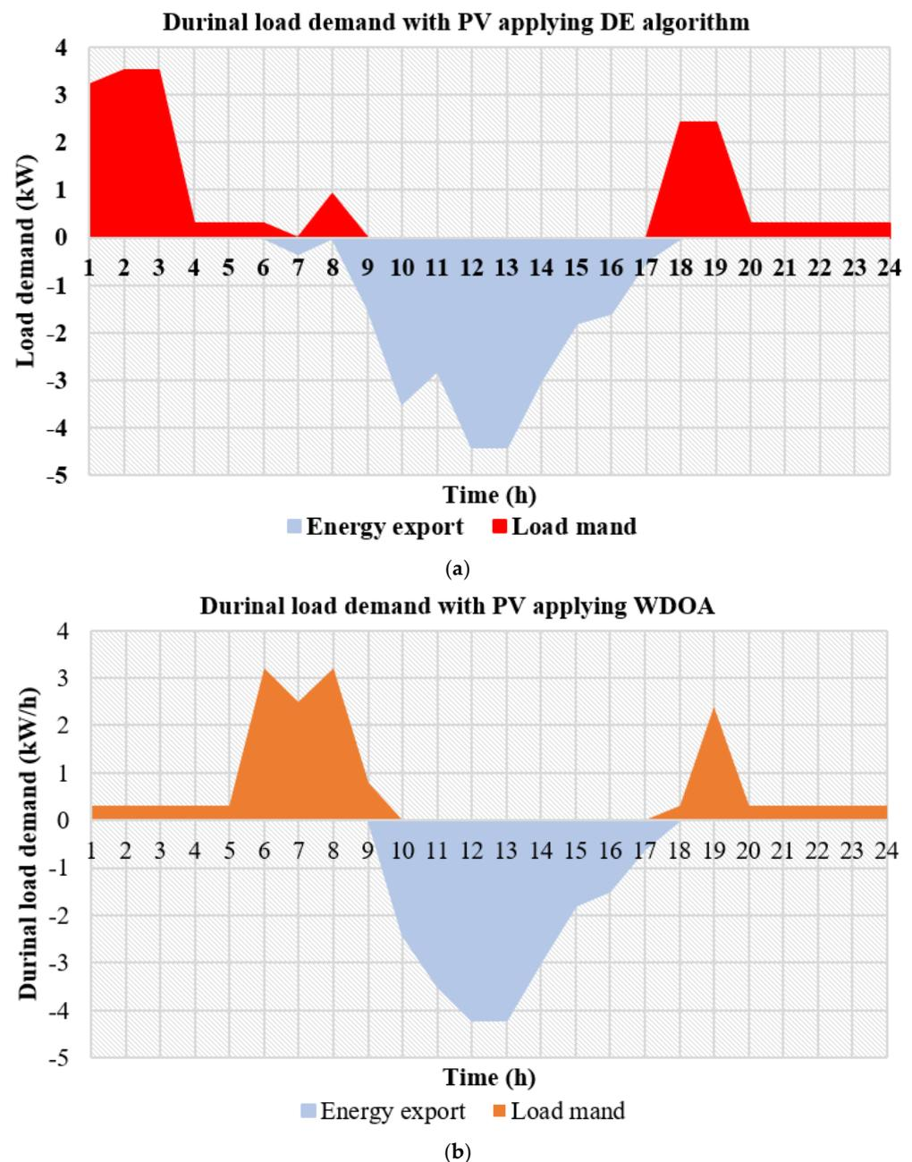
**Figure 9.** The net load demand pattern per day using PV production in order to minimize energy price with restricted time-range planning; (a) DE algorithm; (b) WDOA.
