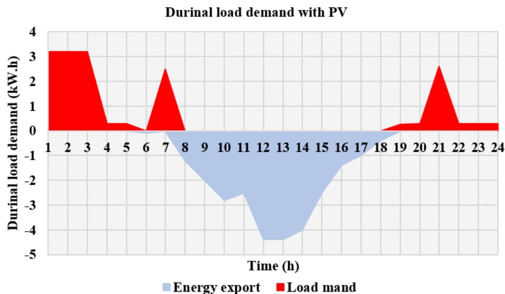
**Figure 7.** Net load profile pattern per day using PV energy with constant time planning.
