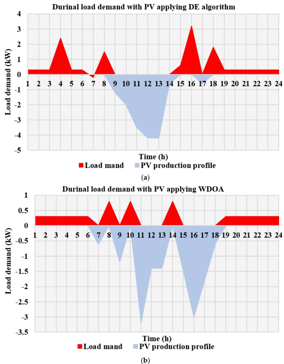
**Figure 11.** The net load profile pattern per day of ScLAs using PV power production with variable time planning; (a) DE algorithm; (b) WDOA.
