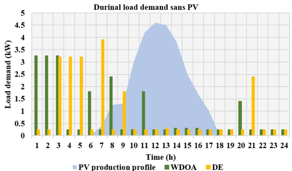
Figure 4. Load pattern per day within restricted time planning and PV production profile.
