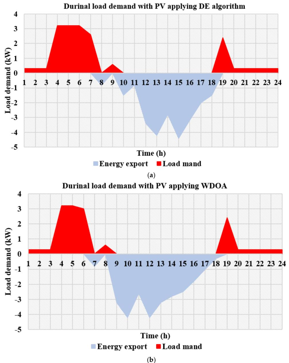
**Figure 10.** The net load demand pattern per day using PV generation in order to minimize energy price with multi-restricted time-range planning; (a) DE algorithm; (b) WDOA.
