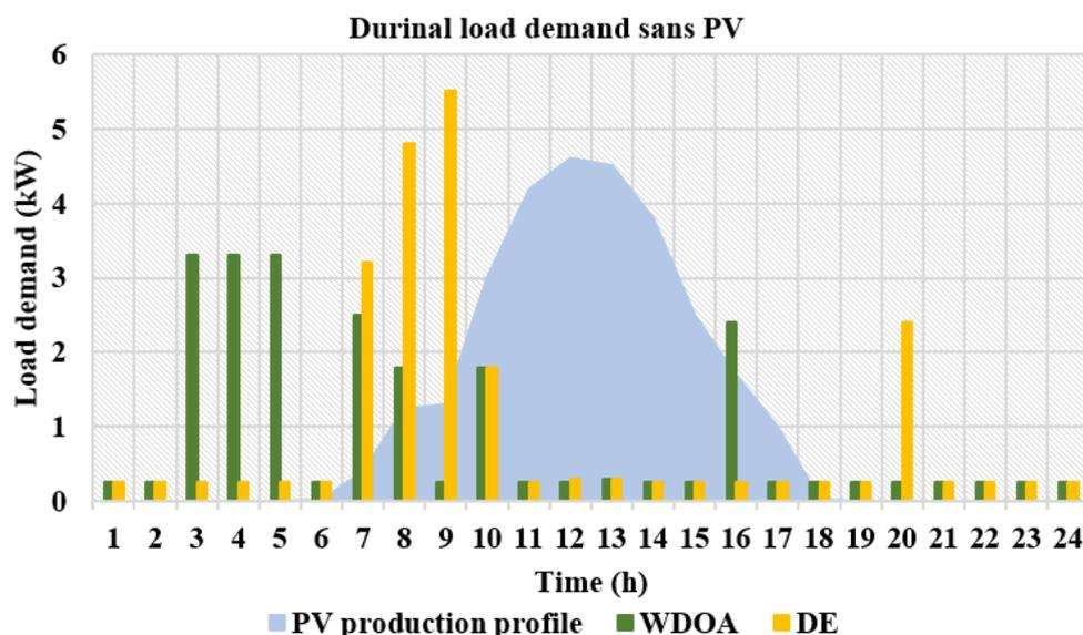
**Figure 5.** Load demand pattern per day with multi-restricted time planning and demonstrating PV production profile.
