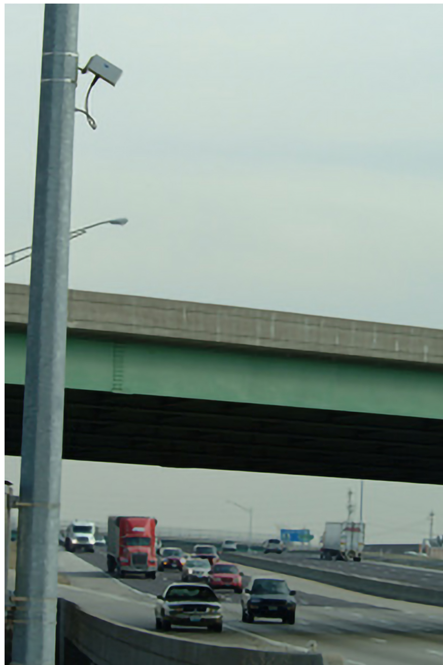
Figure 2. Side-fired microwave radar traffic detector [23].
