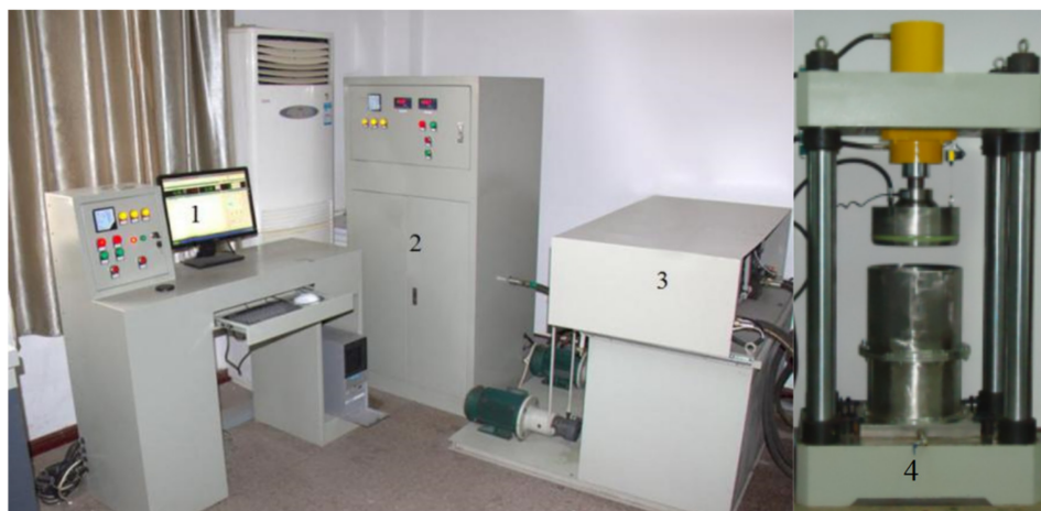
Figure 2. Testing system. 1—Console. 2—Hydraulic pressure double control servo system. 3—Displacement stress double control servo system. 4—Loading system.
