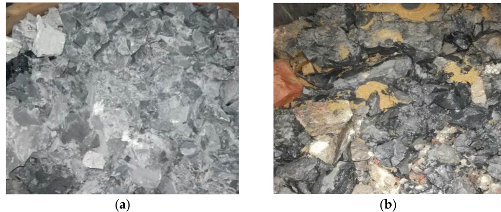
Figure 13. Morphology of broken rocks: (a) natural state; (b) saturated state.
