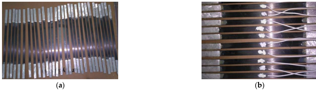
Figure 2. Photographs of the coupons: (a) CFRP plate coupon; (b) location of strain gauge.
