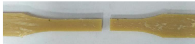
Figure 11. Failure mode of the epoxy adhesive coupon under tension.
