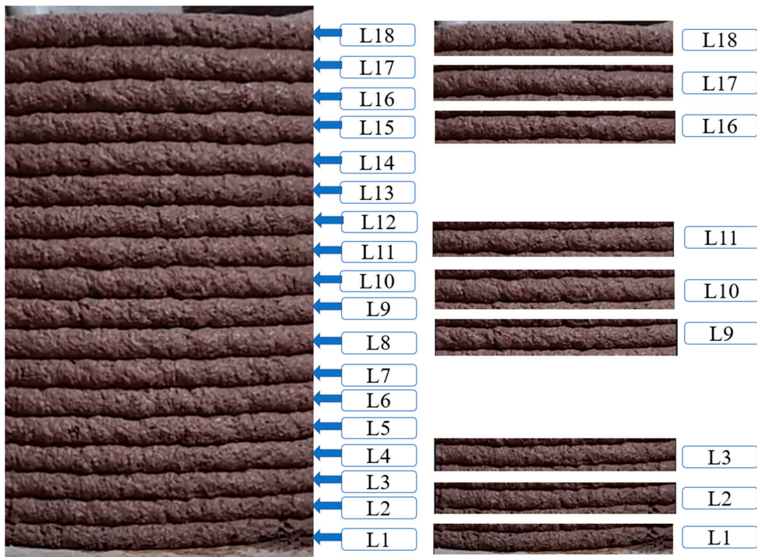
Figure 7. Element A—individual layer designation and a sample representation of the individual—cropped layers subjected to texture analysis.
