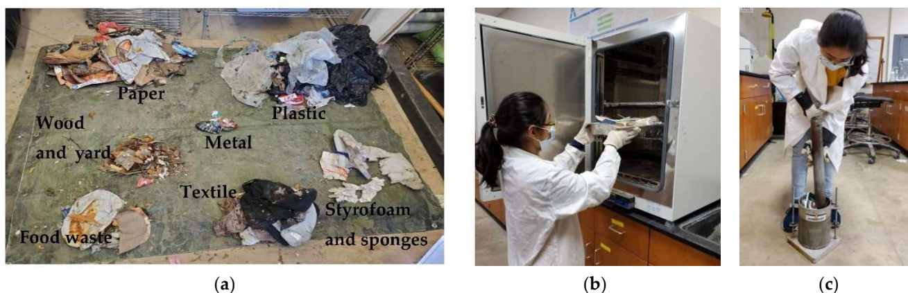
Figure 4. (a) MSW characterization. (b) Moisture content test. (c) Compacted unit weight test.
