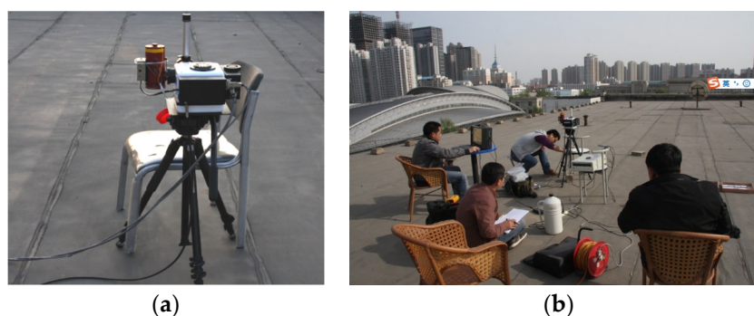
Figure 3. Photos of experimental instruments and experimental sites: (a) Turbo FT thermal infrared spectrometer; (b) site of observation with Turbo FT thermal infrared spectrometer.
