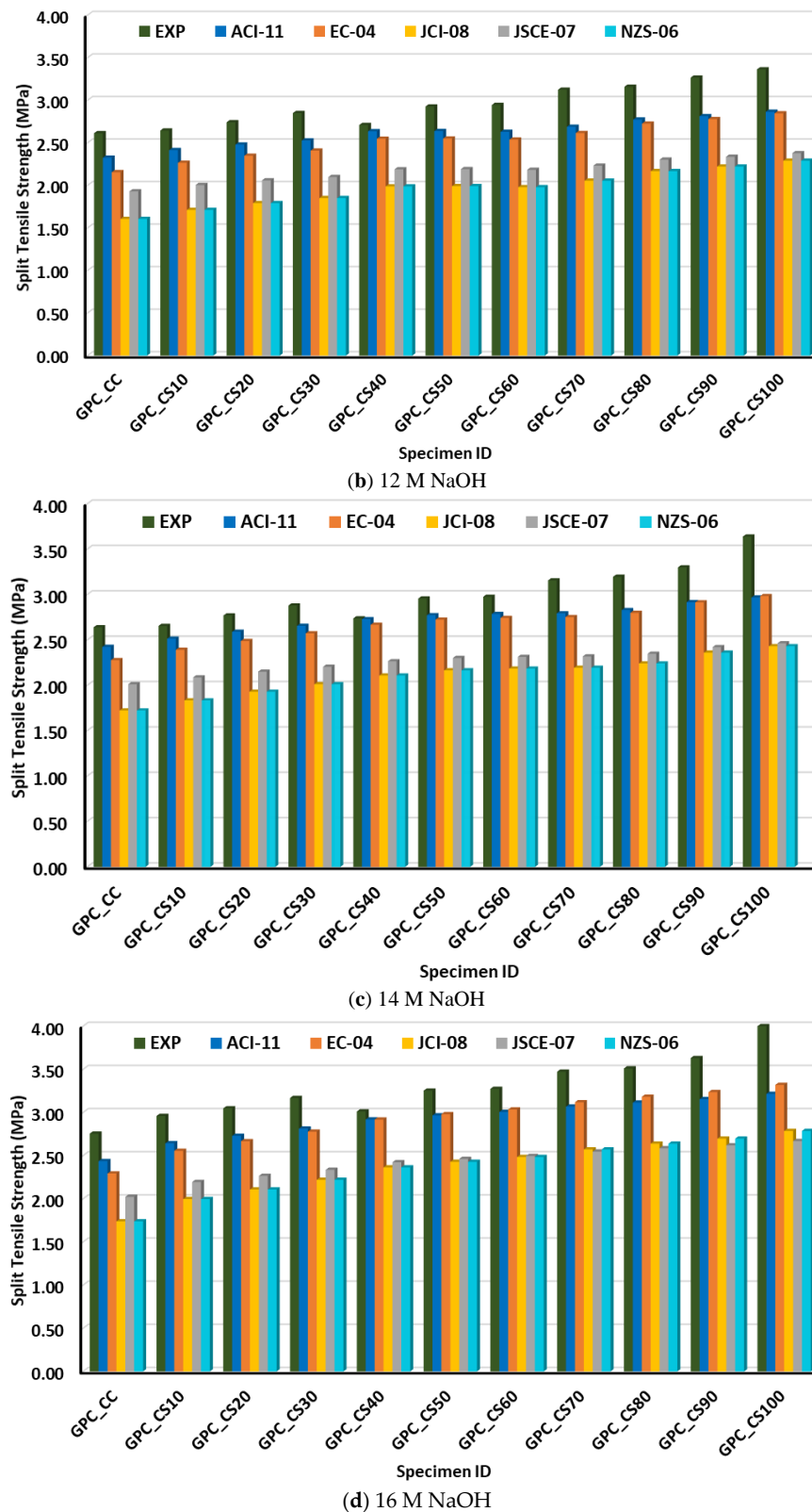
Figure 7. Comparison of split tensile strength results for different molarity levels of NaOH.
