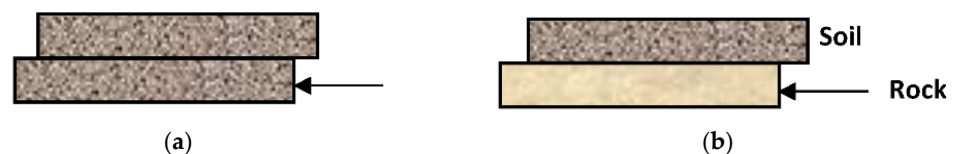
Figure 4. Direct shear test for (a) soil–soil interface resistance and (b) soil–rock interface resistance.
