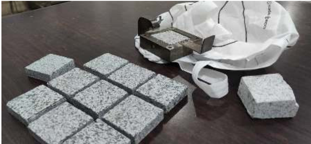
Figure 3. The cut pieces of rock blocks for direct shear tests of soil–rock interface resistance.
