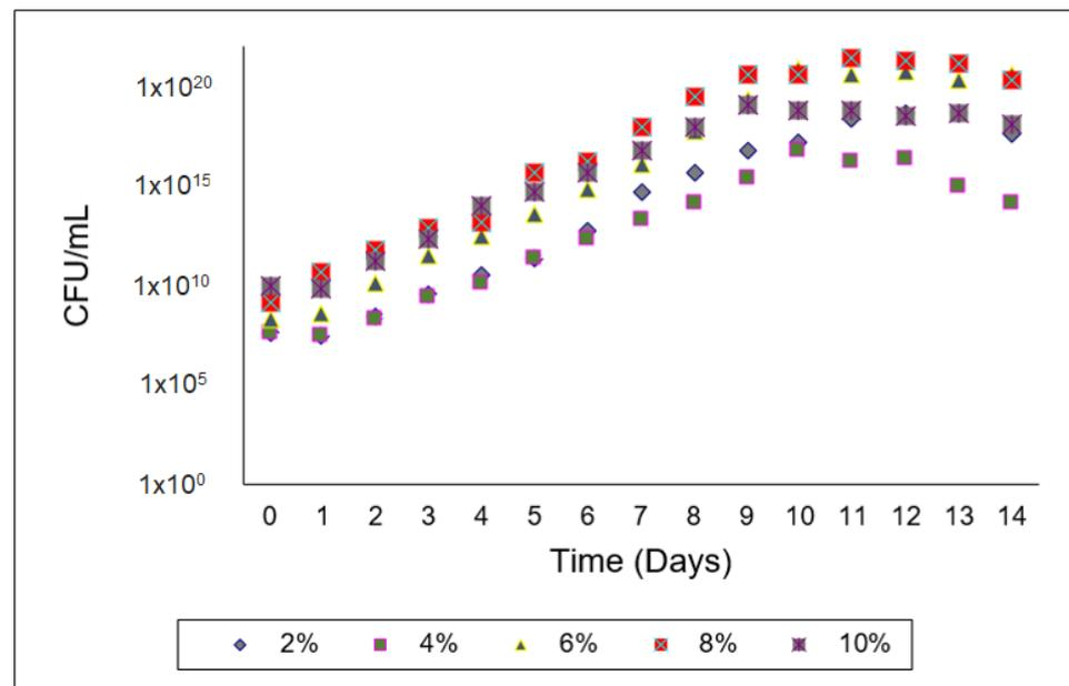
**Figure 2.** Variation profile of microbial biomass when using different concentrations of inoculum from the BIO.PD001 microbial consortium, in the degradation of Diesel 2, in an aerated and stirred bioreactor.
