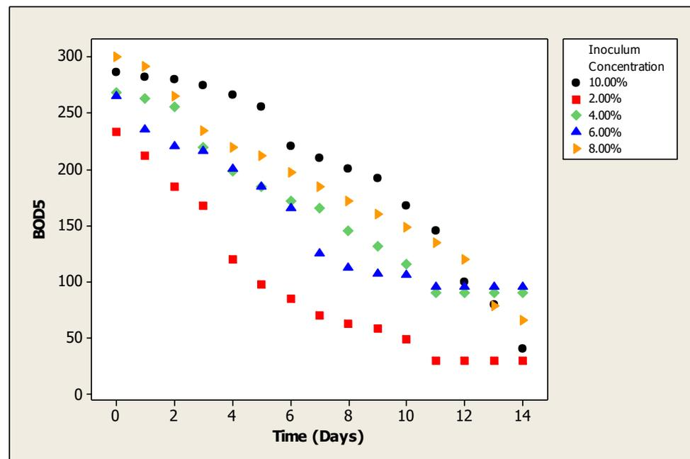
**Figure 3.** Profile of the variation of the Biochemical Oxygen Demand (BOD<sub>5</sub>) when using different concentrations of inoculum of the BIO.PD001 microbial consortium, in the degradation of Diesel 2, in an aerated and stirred bioreactor.
