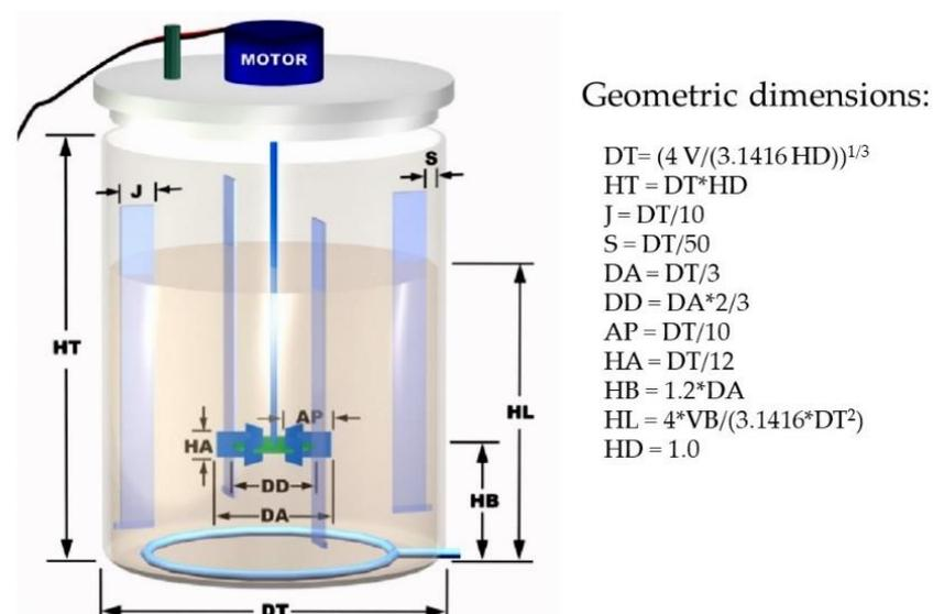
Figure 1. Stirred tank Bioreactor design.
