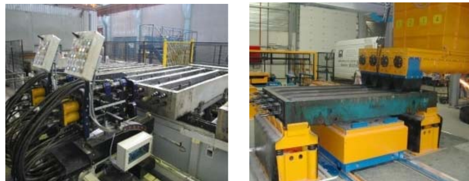
Figure 13. Tensioning and concrete pouring of concrete of pre-tensioned short-mould flow method.
