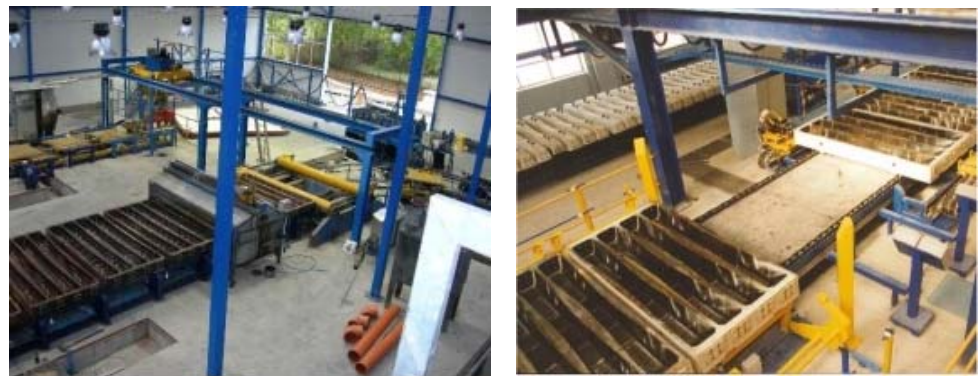
Figure 12. Overview of the production line of pre-tensioned short-mould flow method.
