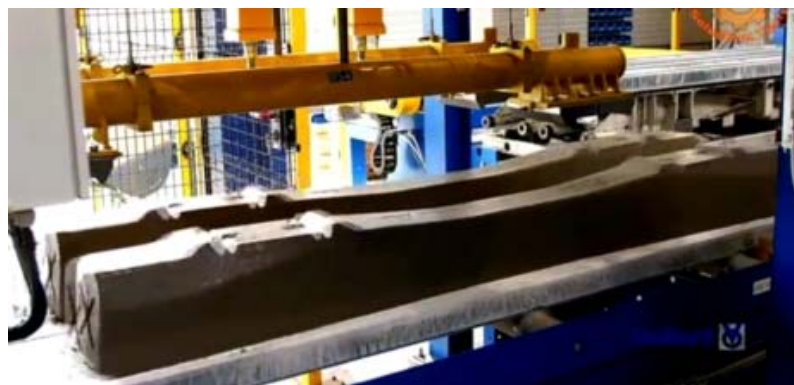
Figure 21. Instant-demoulded short-mould flow method demoulding process.
