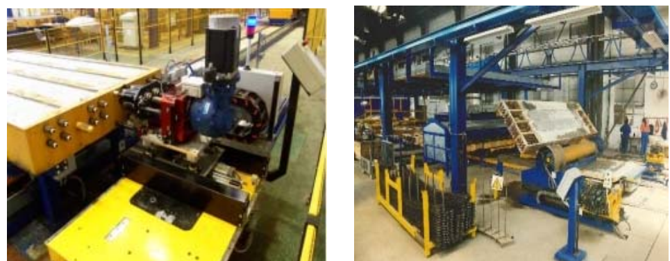
Figure 14. Transmitting and demoulding of pre-tensioned short-mould flow method.
