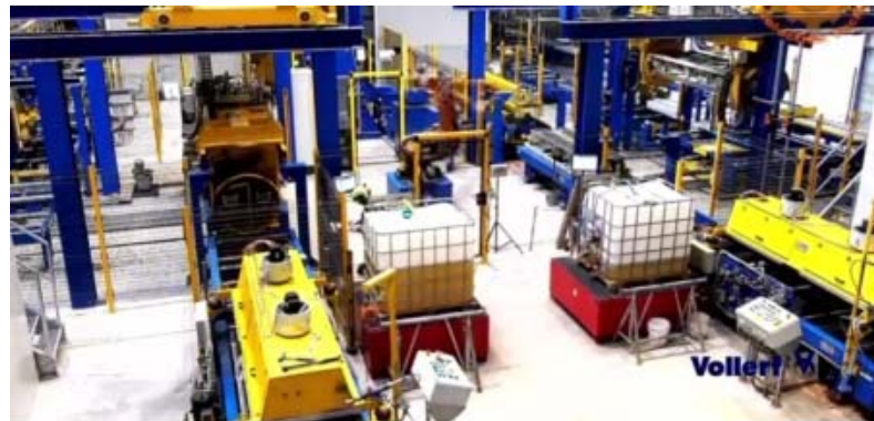
Figure 20. Overview of the production line of instant-demoulded short-mould flow method.
