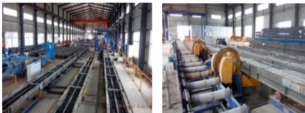
Figure 8. Overview of production line of long-mould flow method.
