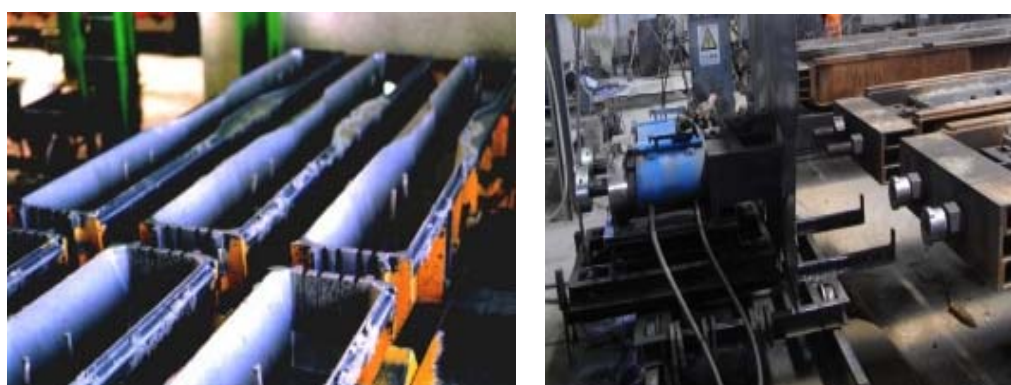
Figure 9. Long-mould flow method mould and tension process.
