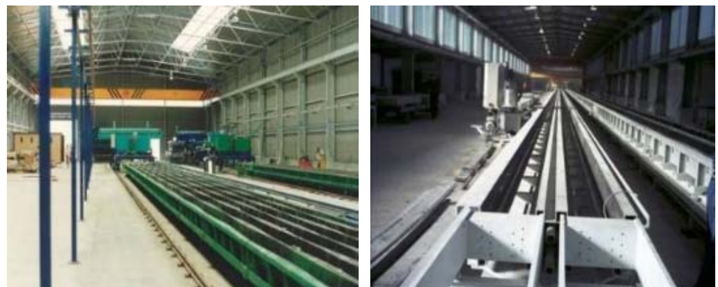
Figure 4. Overview of long-line system method production plant.
