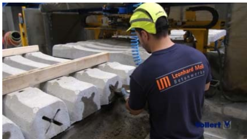
Figure 18. Sealing anchor for post-tensioned short-mould flow method.
