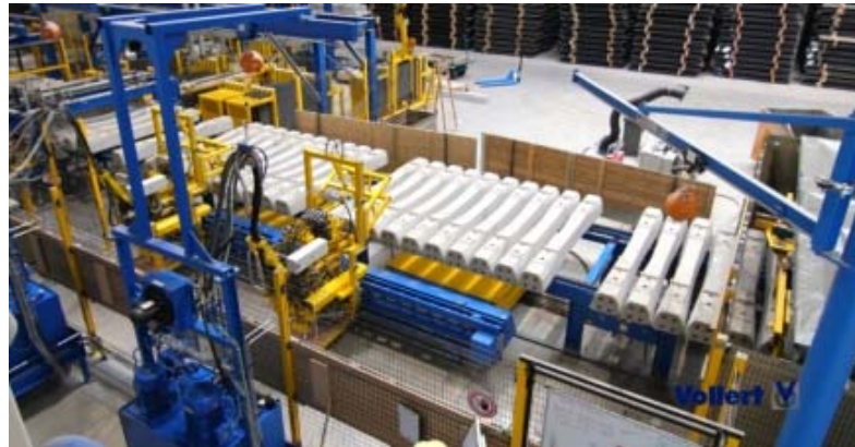
Figure 16. Overview of the production line of post-tensioned short-mould flow method.
