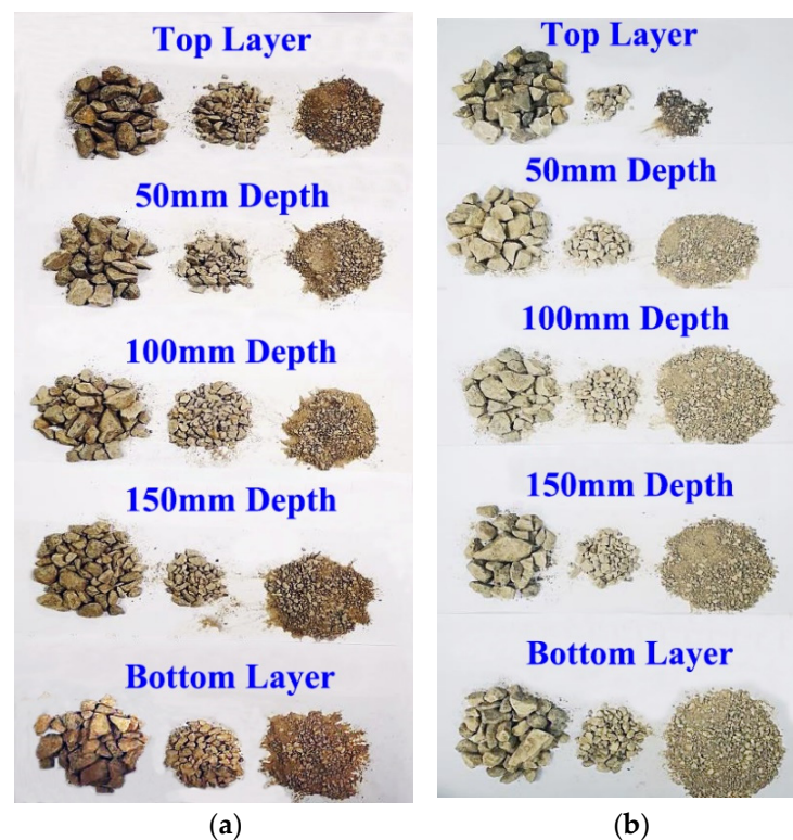
Figure 9. Sieve results of aggregate at different depths before and after infiltration; (a) the initial state; (b) after infiltration.
