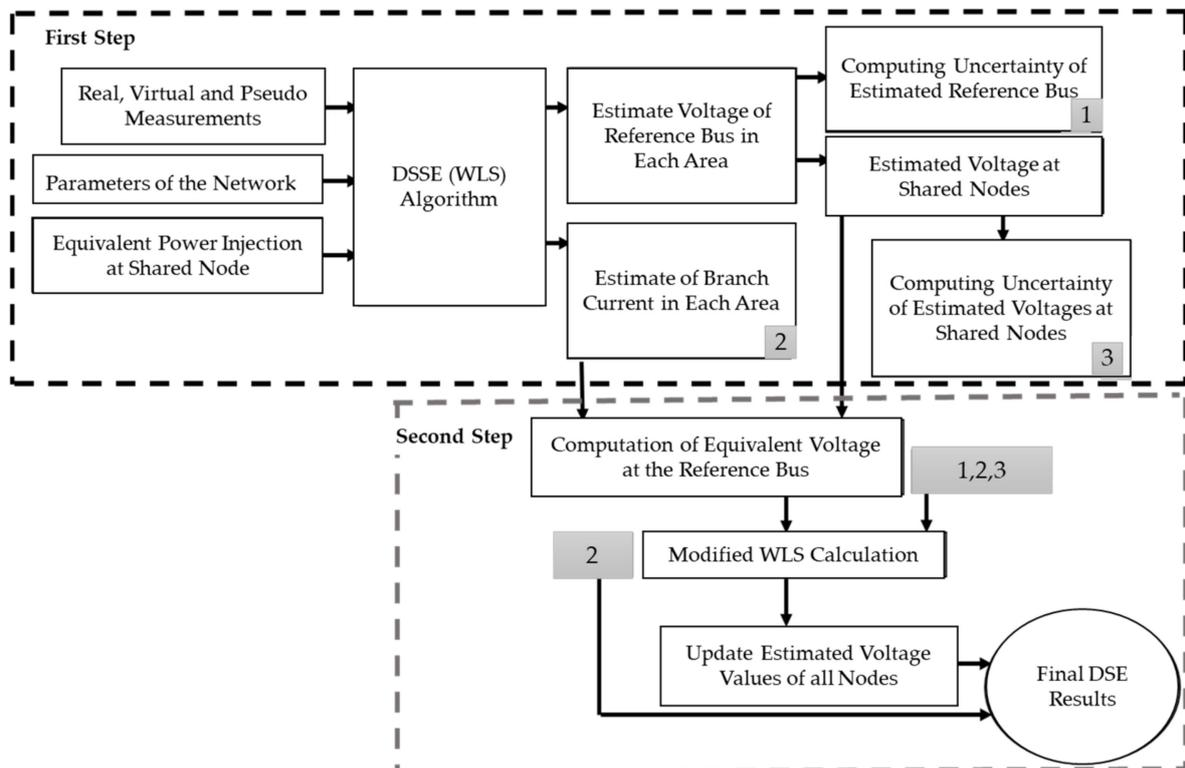
Figure 6. Two-step of DS-DSE procedures.
