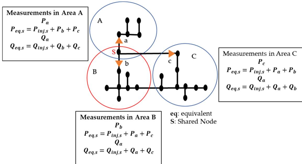
Figure 5. Equivalent Measurements at shared nodes for three sub-areas.
