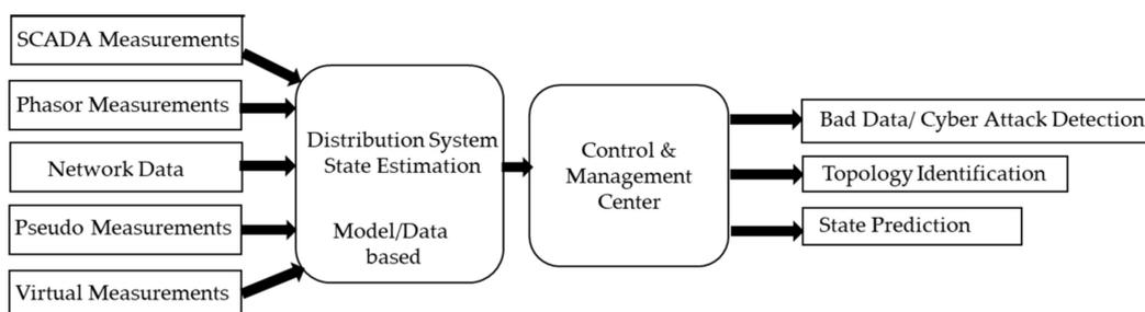
**Figure 1.** Overview of State Estimation in Distribution Networks.
