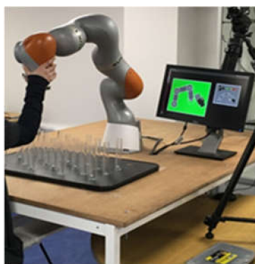
Figure 3. KUKA iiwa and experimental task setup. On the screen, graphics are displayed indicating permitted interaction.
