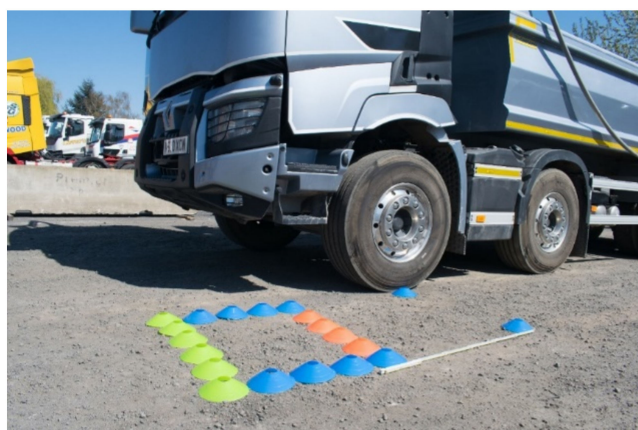
Figure 12. Marker cones for testing forward coverage.
