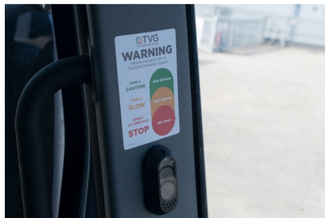
Figure 8. Warning lights and buzzer.
