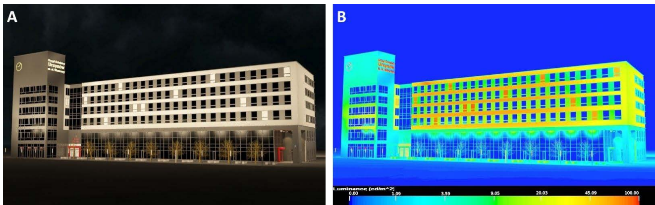
Figure 11. Modern building floodlighting with the planar method: (A)—visualization, (B)—luminance distribution.
