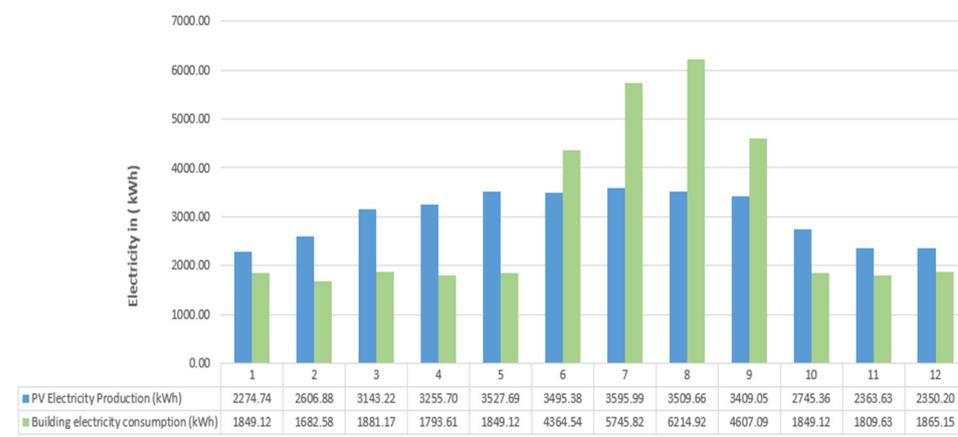
**Figure 9.** PV Electricity Production vs. Building Electricity Consumption.
