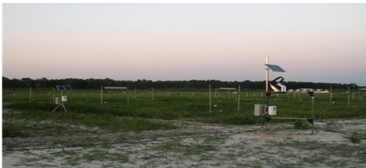
Figure 3. Long-term monitoring layout. The instruments used are heat flux recorder, pyranometer recorder, soil temperature and humidity probe, air temperature and humidity probe, and evaporation pan.
