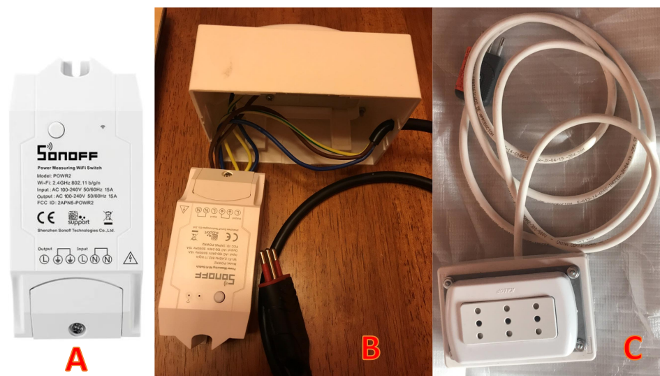
Figure 13. Equipment for Data Acquisition stage: Sonoff Pow R2 (A) and customized version used as smart plug (B,C).
