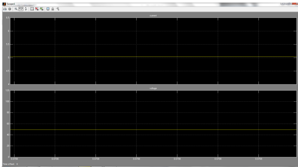
Figure 5. PV Voltage and Current.
