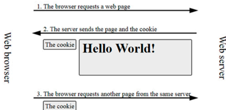
Figure 2. A simple representation of the communication between the cookie and the server [13].
