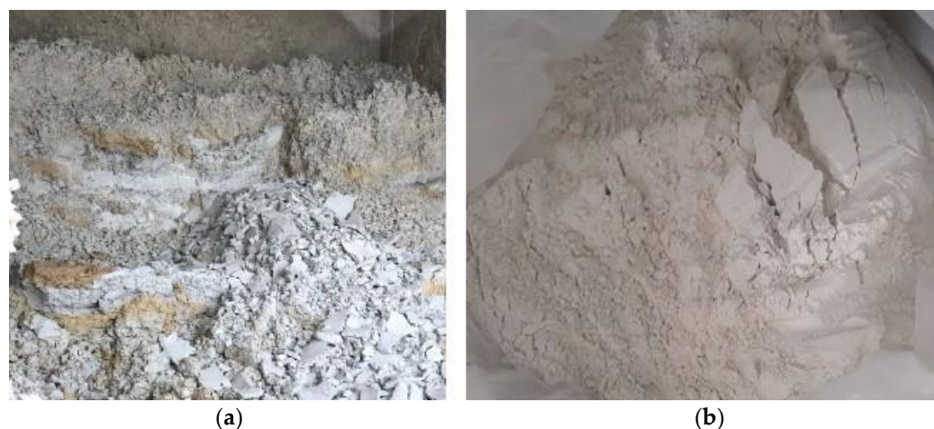
Figure 1. Ornamental Rock Waste (a) in the ornamental rock industry with humidity, (b) dry and passed at #50.
