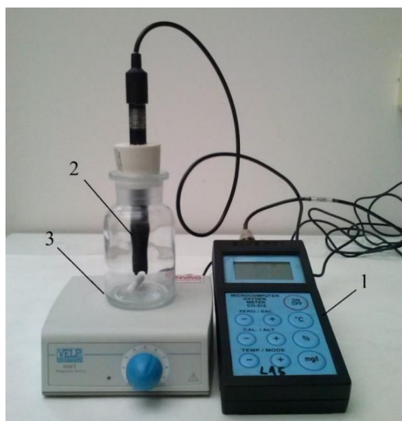
Figure 2. Apparatus for determining the respiratory activity of leachate microorganisms (1—oxygen meter; 2—oxygen probe; 3—magnetic stirrer).
