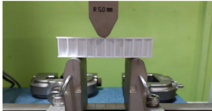
**Figure 8.** Experimental bending test setup.
