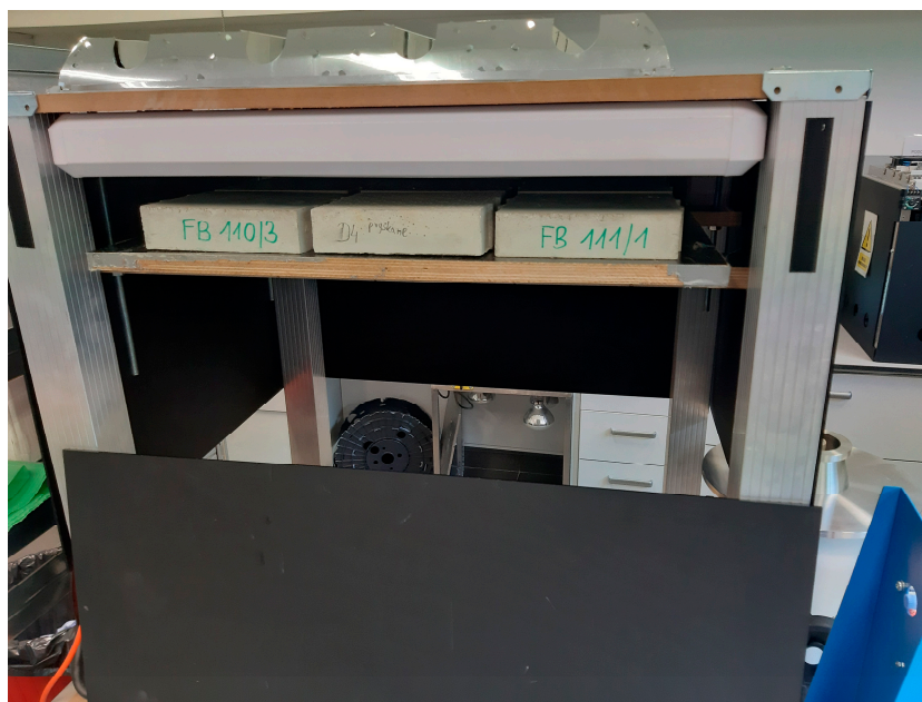
Figure 11. UV-A irradiation chamber with the distance between UV-A lamps and tested surface set in a way that irradiation of UV-A was 10 \text{ W/m}^2 .
