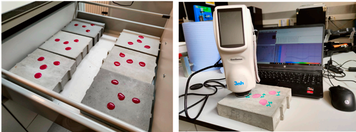
Figure 12. Samples of photocatalytic cementitious mortars with drops of rhodamine and color testing using a spectrophotometer.
