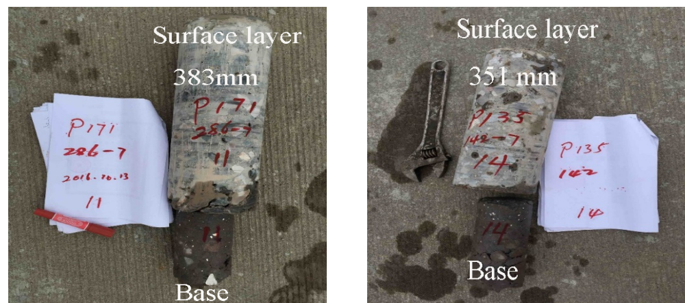
Figure 14. Runway core sampling thickness inspection results.
