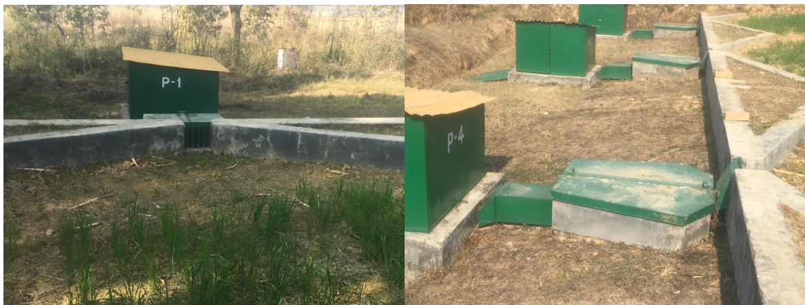
Supplement Figure S10. Two-stage multi-slots devisor with runoff collection tanks
