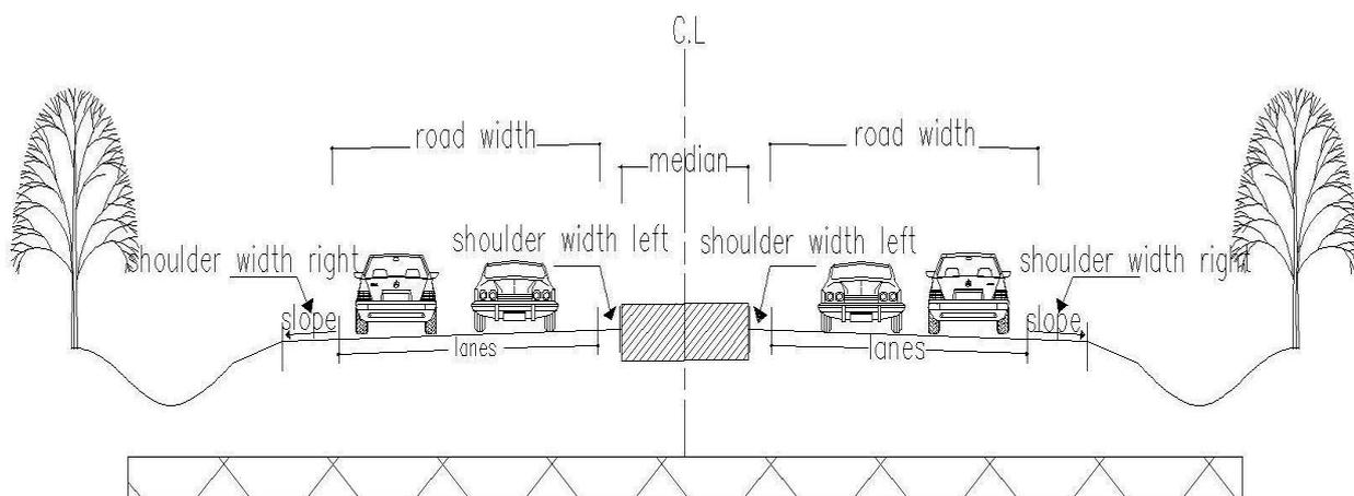
Figure 6. Cross section of road.
