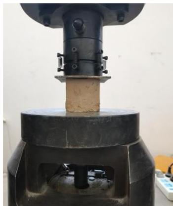
**Figure 2.** Compressive-strength test of the mud test block.
