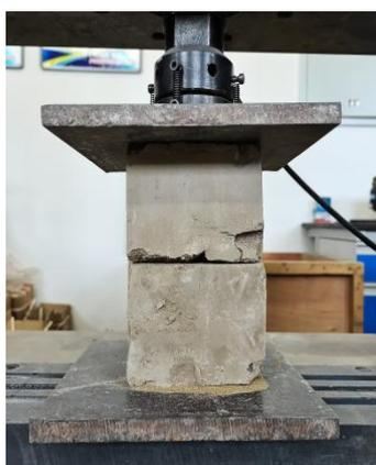
**Figure 3.** Compressive-strength test of the adobe block.
