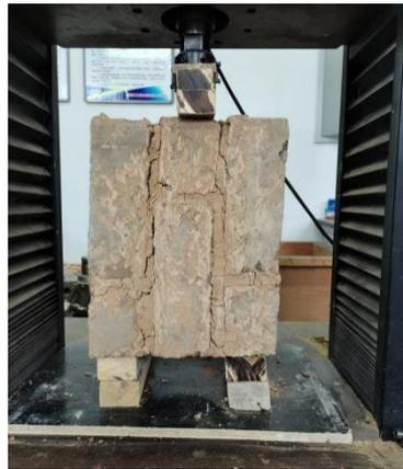
**Figure 4.** Shear-strength test of masonry.
