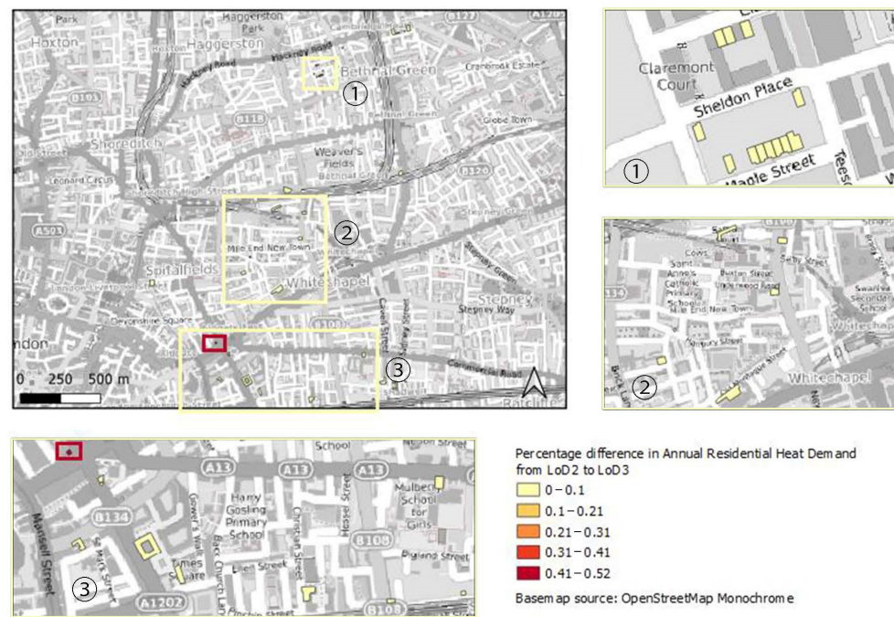
Figure 15. Percentage difference in annual residential heat demand from LoD2 to LoD3 for Area 2.
