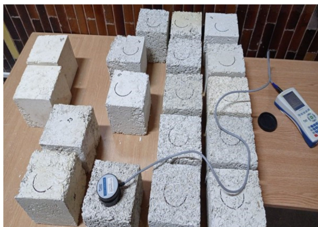
Figure 6. Measurement for the heat transfer coefficient using ISOMET 2114 [60].
