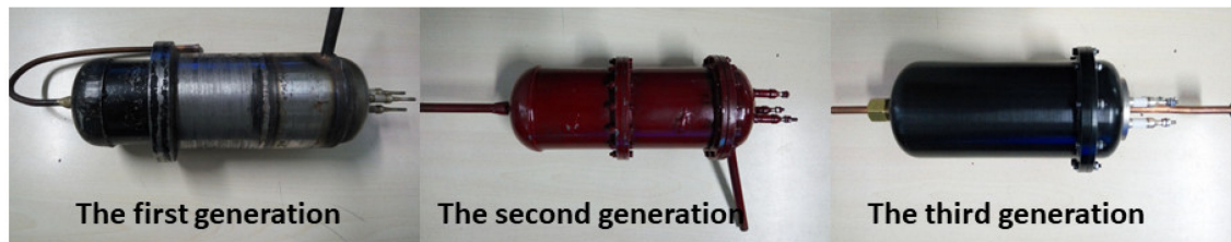
Figure 4. The prototypes of the Wankel compressor.
