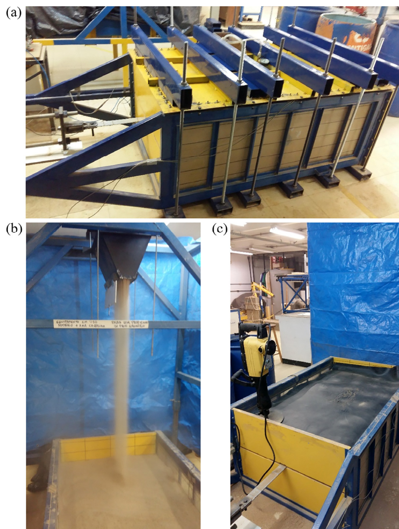
Figure 4. Photographs of the pullout equipment employed in this study: (a) side view of the pullout box, (b) sand rain procedure, and (c) soil compaction using a mechanical hammer.
