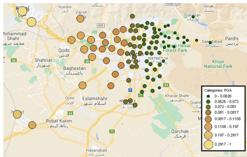
**Figure 7.** Acceleration in bridges, subjected to record No. 1 (magnitude of 7.2 on the Richter scale).
