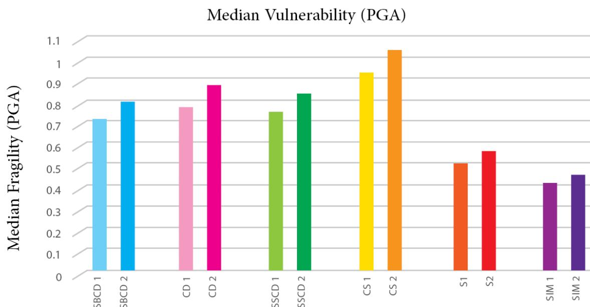
**Figure 23.** Median vulnerability values of different bridge systems with an age of less or more than 10 years.
