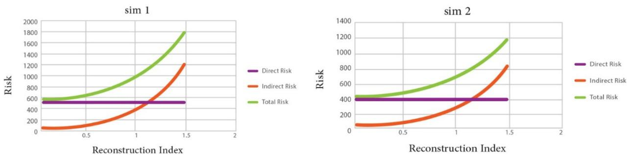
Figure 28. Variations of direct, indirect, and total risk versus changes in the reconstruction index for models sim1 and sim2.
