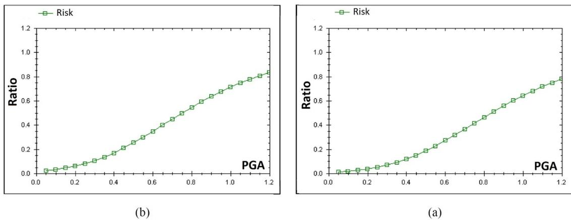
**Figure 19.** Risk functions of concrete slab–steel box bridge aged (a) less than 10 years, and (b) more than 10 years.
