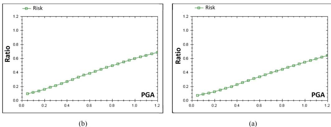
**Figure 18.** Risk functions of concrete slab bridge aged (a) less than 10 years, and (b) more than 10 years.
