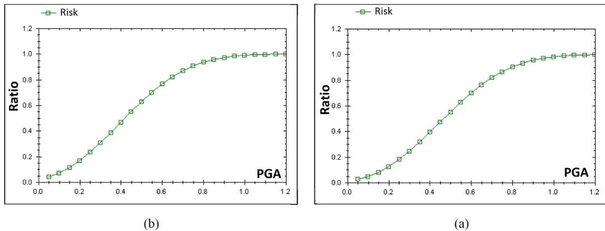
**Figure 22.** Risk functions of simple bridge aged (a) less than 10 years, and (b) more than 10 years.
