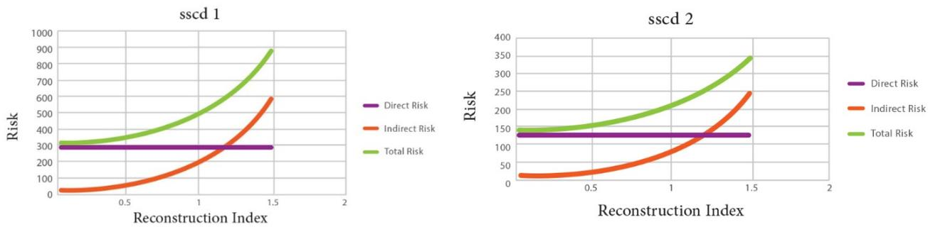
Figure 27. Variations of direct, indirect, and total risk versus changes in the reconstruction index for models sscd1 and sscd2.
