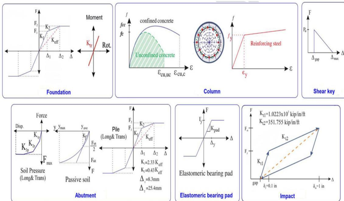
Figure 13. Non-linear responses of various bridge components modeled in OpenSEES [6].
