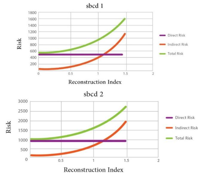
Figure 26. Variations of direct, indirect, and total risk versus changes in the reconstruction index for models sbcd1 and sbcd2.
