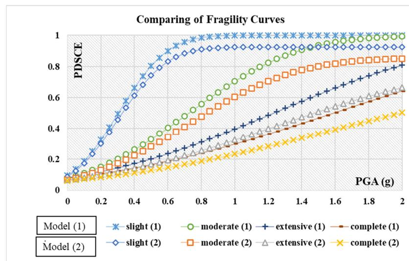
**Figure 14.** Comparison of the fragility curve results between model (1): obtained from decision tree analysis and model (2): extracted from IDA modeling.
