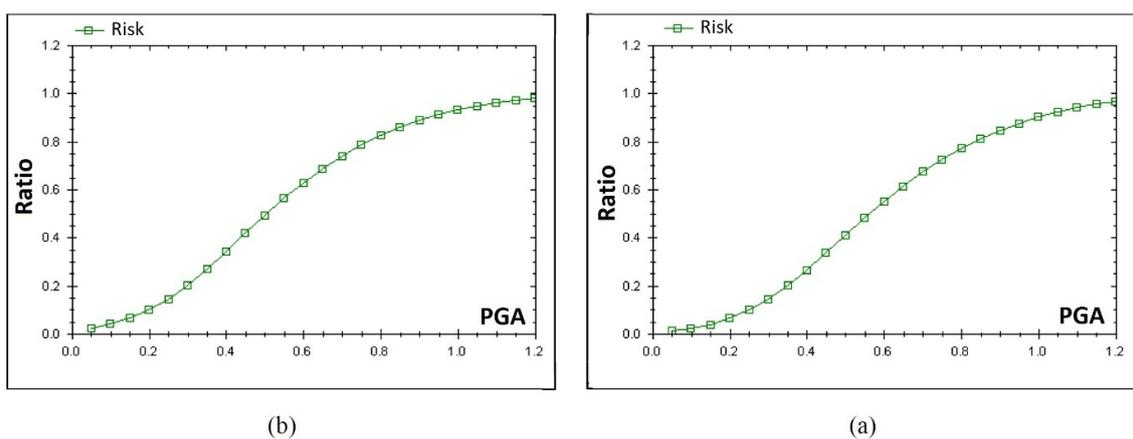
**Figure 21.** Risk functions of steel bridge aged (a) less than 10 years, and (b) more than 10 years.
