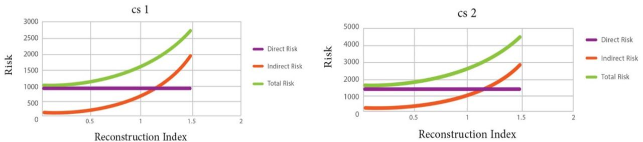
**Figure 30.** Variations of direct, indirect, and total risk versus changes in the reconstruction index for models cs1 and cs2.
