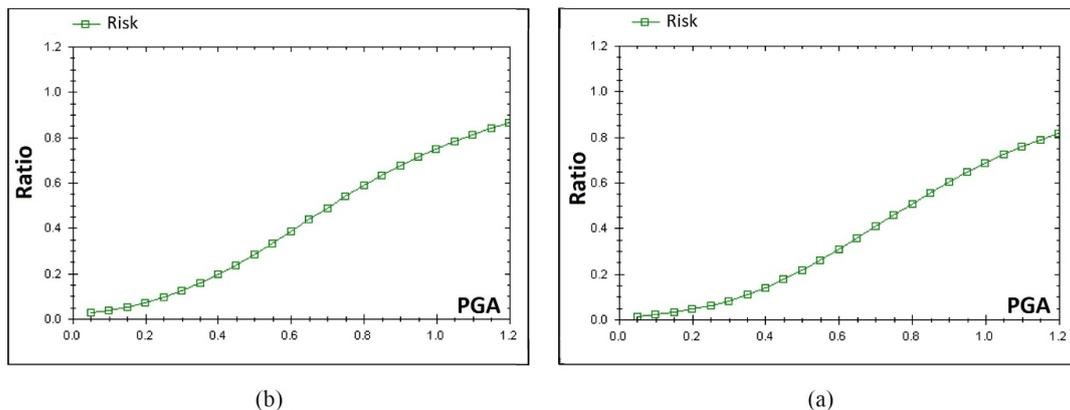
**Figure 17.** Risk functions of concrete slab box bridge aged (a) less than 10 years, and (b) more than 10 years.
