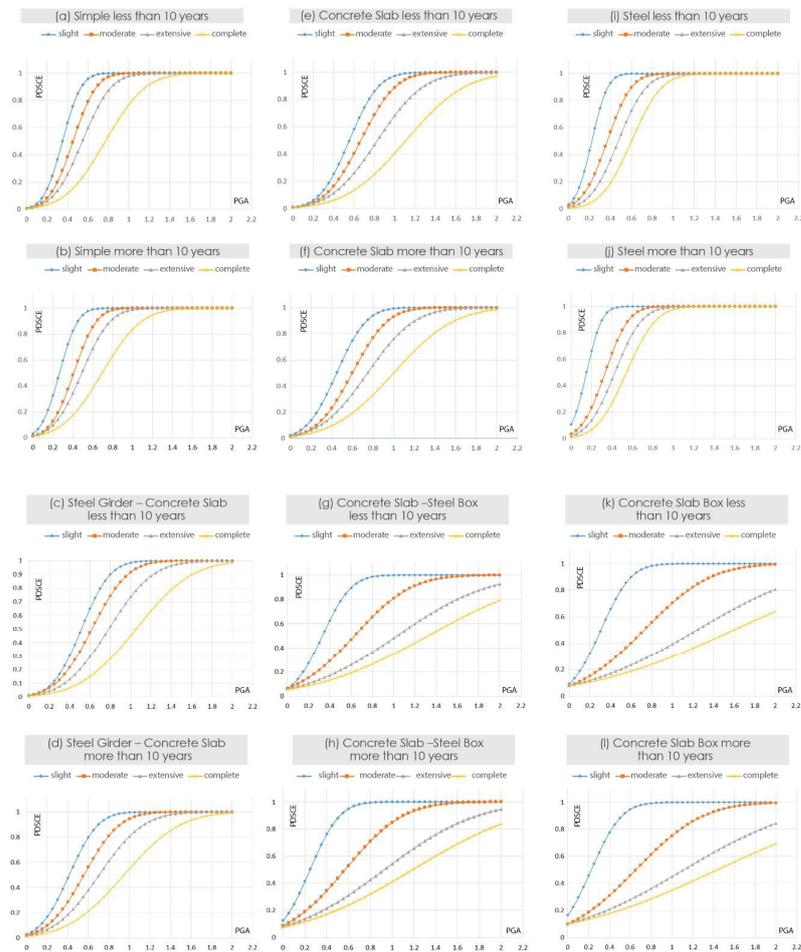
**Figure 10.** Fragility curves for different bridge systems at different ages and various damage states [66].
