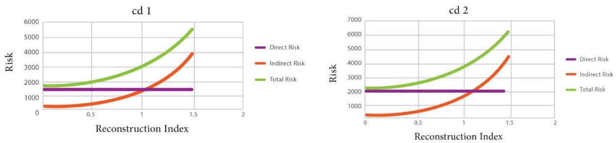
**Figure 29.** Variations of direct, indirect, and total risk versus changes in the reconstruction index for models cd1 and cd2.
