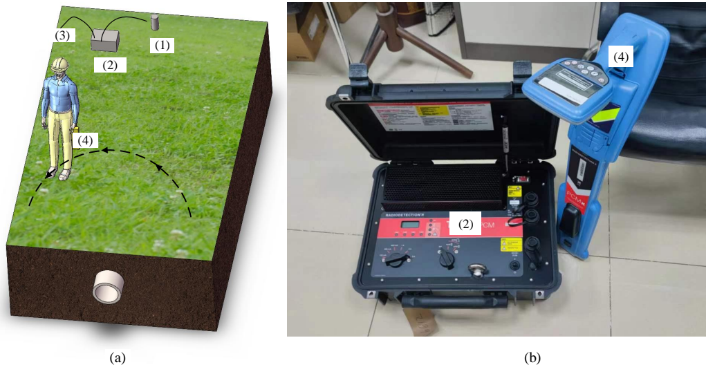
Figure 2. The device and principle of PCM. (a) The principle of PCM. (b) The practical device called a PCM. Here, (1) represents the pipeline test pile, (2) represents the high-power signal transmitter, (3) represents the transmitter's ground point, and (4) represents the PCM receiving equipment.
