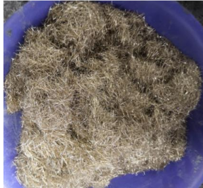
Figure 7. Extra-fine steel fiber for the tests.
