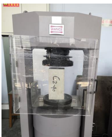
Figure 4. Test of axial compressive strength.
