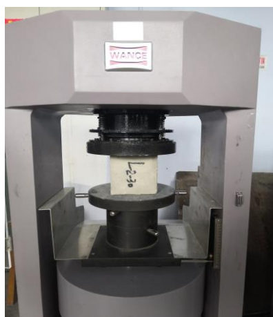
Figure 3. Test of cubic compressive strength.
