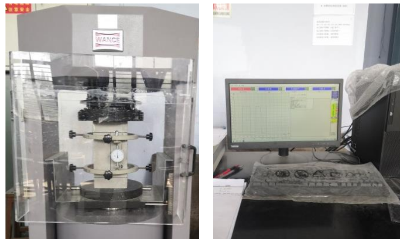
Figure 6. Process for the elastic modulus test.
