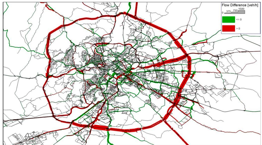
**Figure 5.** Comparison of link flows due to the presence of AVs (50% AVs with respect to 0% AVs).
