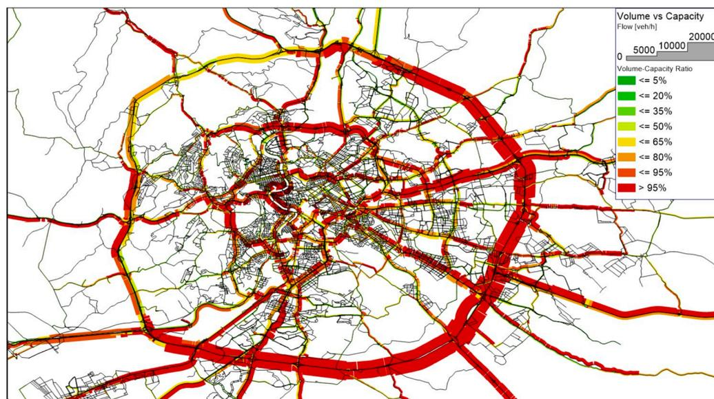
**Figure 1.** Example of assignment results: link flows and volume–capacity ratios (50% AVs).
