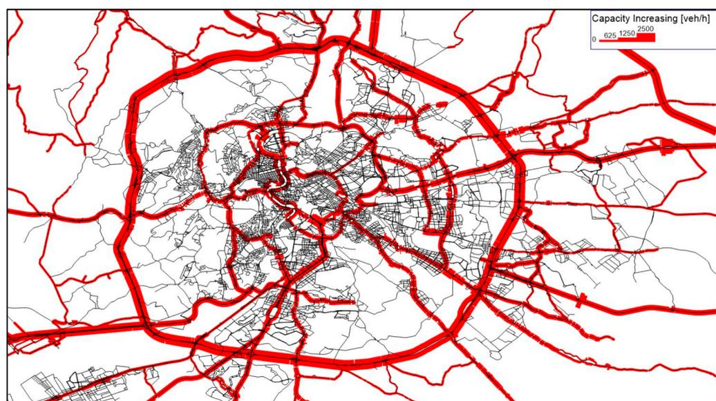
**Figure 2.** Example of assignment results: link capacity increasing (50% AVs).
