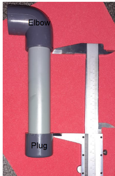
Figure 6. The base of the antenna, which is made up of the PVC tube and has the elbow and the plug mounted; recall that the space must be 10 cm.
