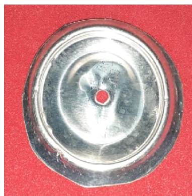
Figure 10. Base of the can that will go at the end of the antenna.
