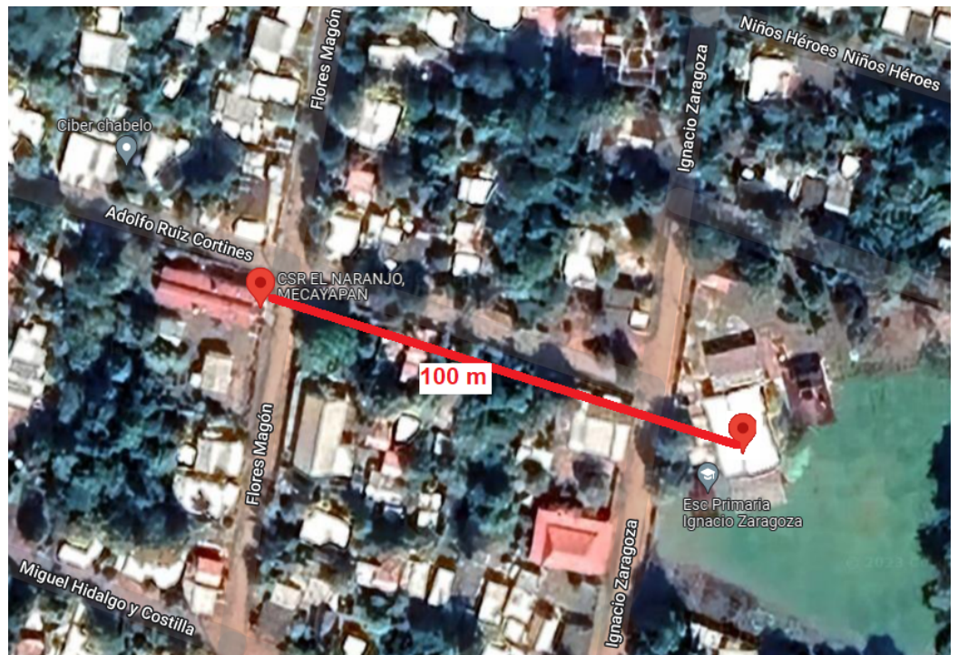
Figure 15. Coverage distance with the antenna connected from community health center to the Ignacio Zaragoza Elementary School.
