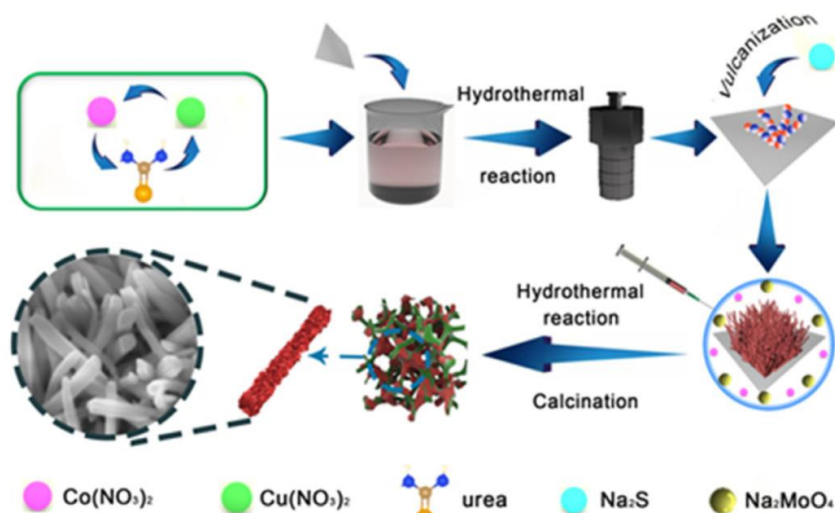
Scheme 2. Illustration of the synthesis of the \text{CuCo}_2\text{S}_4/\text{CoMoO}_4 nanorod array on the NF substrate. Reprinted with permission Ref. [64] with permission license 5536080833324. Copyright Elsevier. 25 April 2023.
