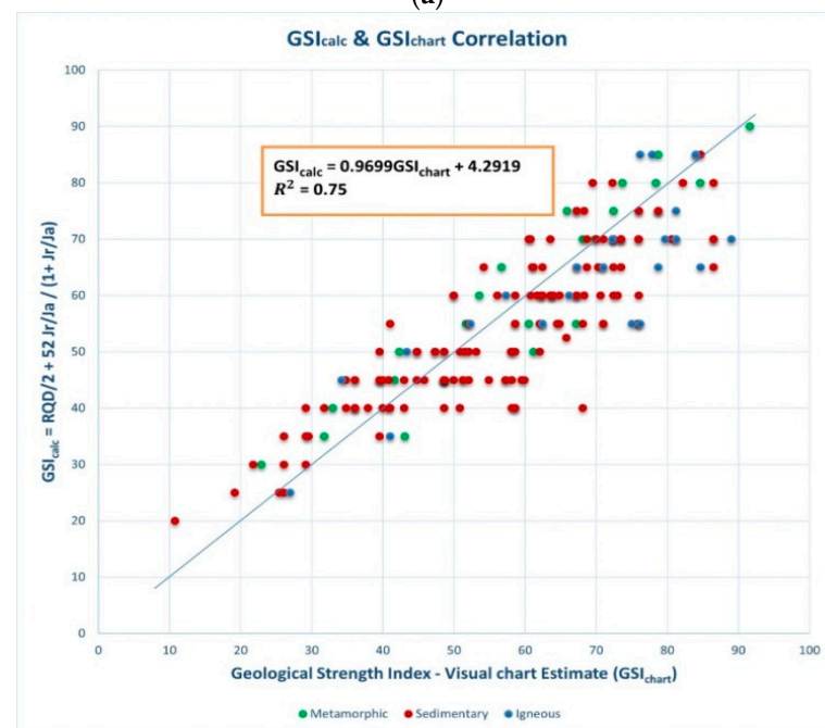
Figure 9. Relationships between GSI_{chart} and GSI_{2013} : (a) separated for igneous, sedimentary, meta-morphic rocks, (b) for all rocks.
