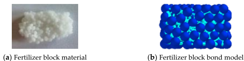
Figure 5. Fertilizer block material and bond model.
