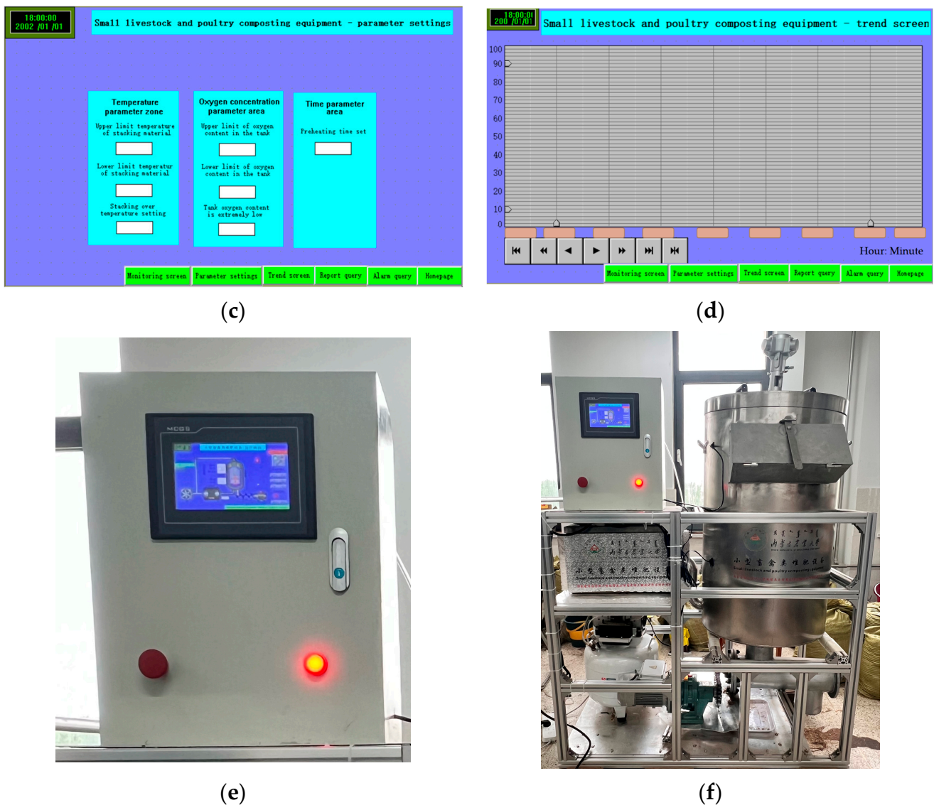
Figure 11. Normal operation of the control section. (a) Login screen; (b) Monitoring screen; (c) Parameter settings; (d) Trend screen; (e) External control box; (f) Improved composting equipment entity.
