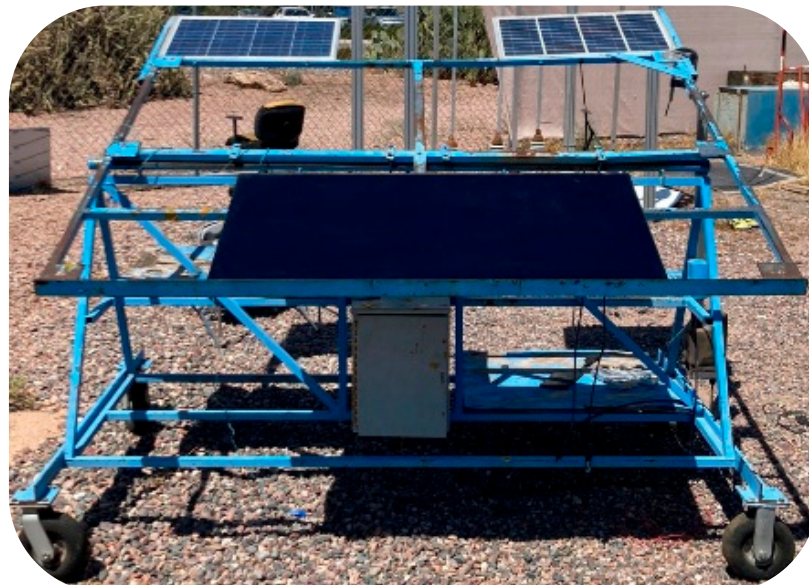
Figure 2. Illustration of a module under hotspot test outdoors on a two-axis tracker.
