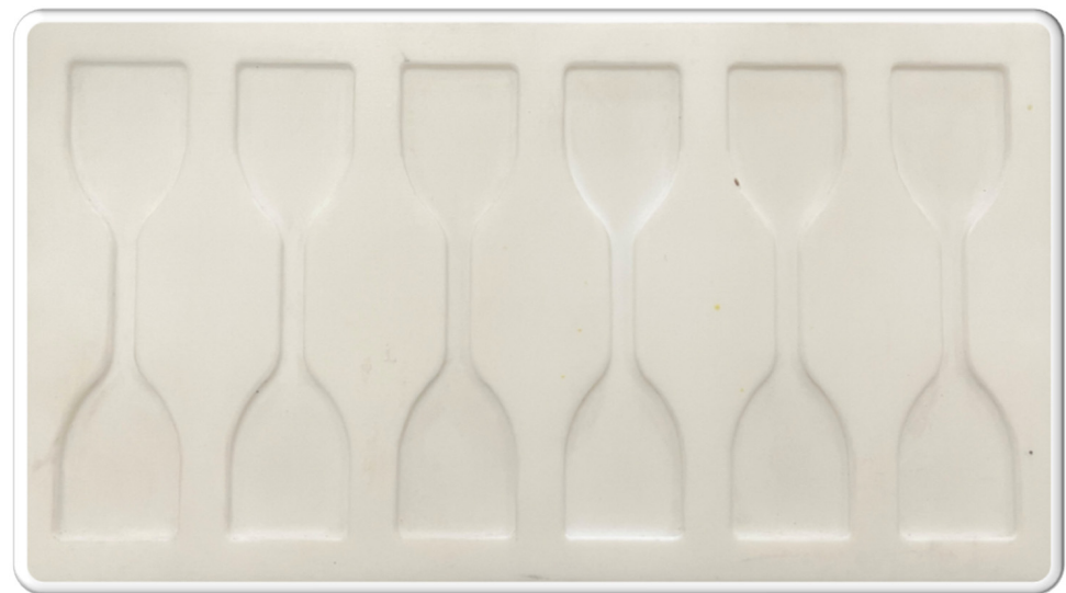
Figure 4. The mold for tensile property experiment.
