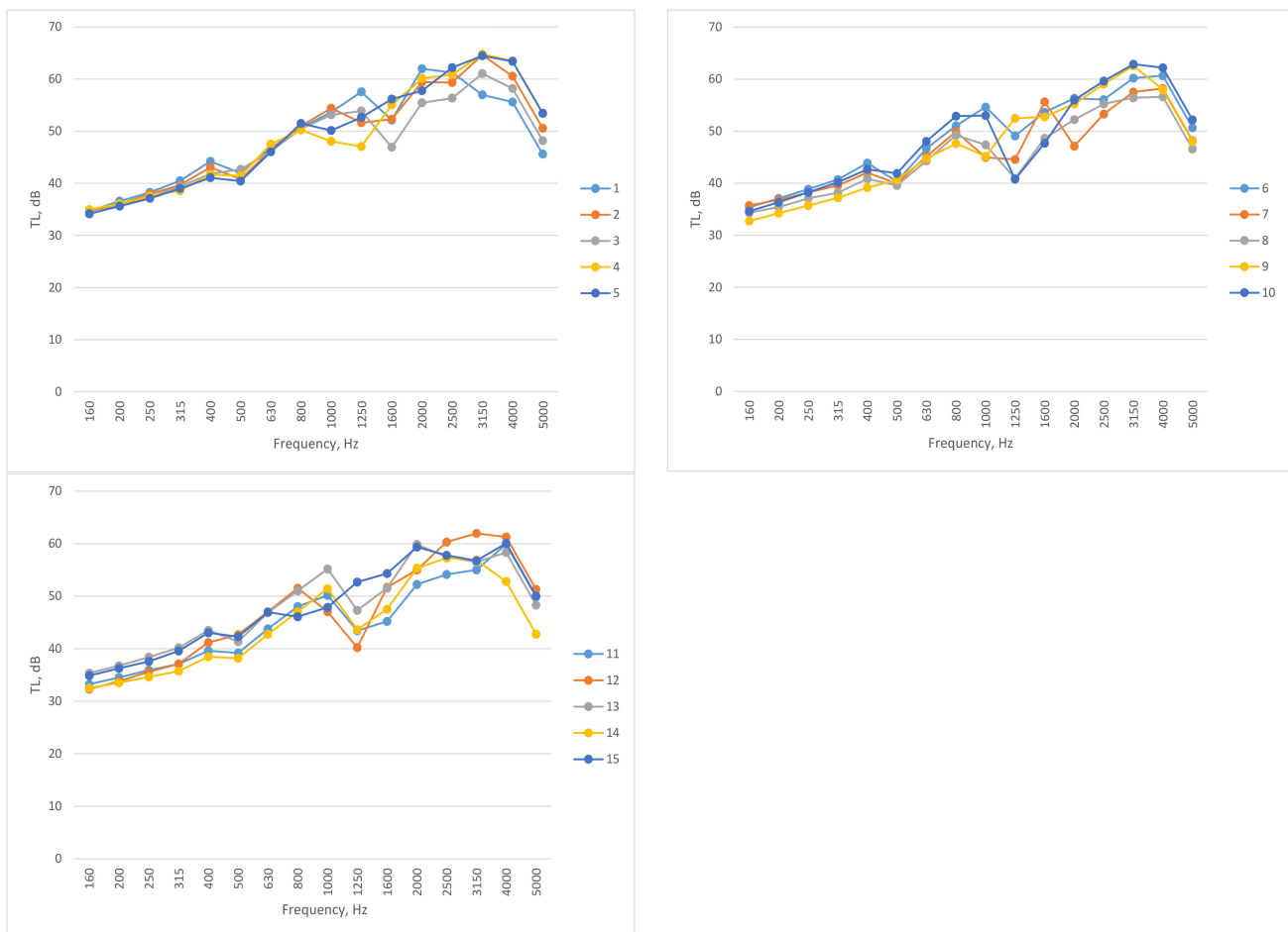
Figure 9. Experimental results of transmission loss measurements of 12 \pm 2 mm thickness rubber sample with plasterboards (GKFI) on both sides.
