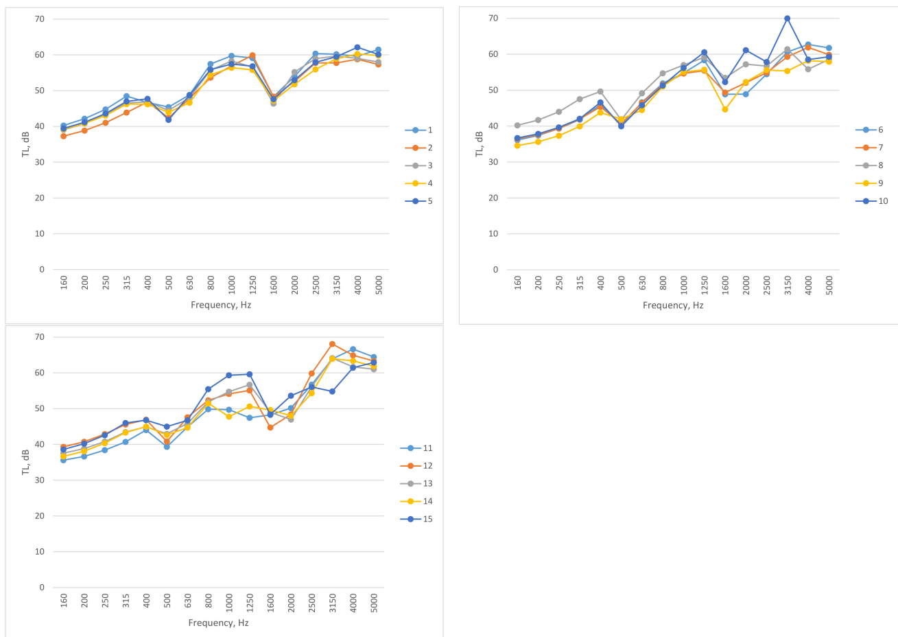
Figure 11. Experimental results of transmission loss measurements of 25 \pm 2 mm thickness rubber sample with plasterboards (GKFI) on both sides.
