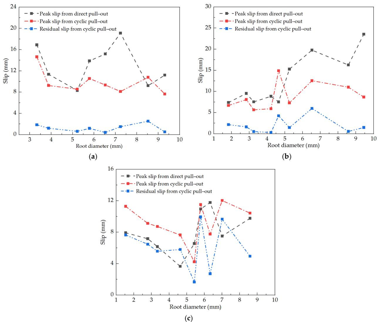
**Figure 11.** Comparison of characteristic slip under different cyclic loading amplitudes. (a) At 25% cyclic loading amplitude. (b) At 50% cyclic loading amplitude. (c) At 75% cyclic loading amplitude.
