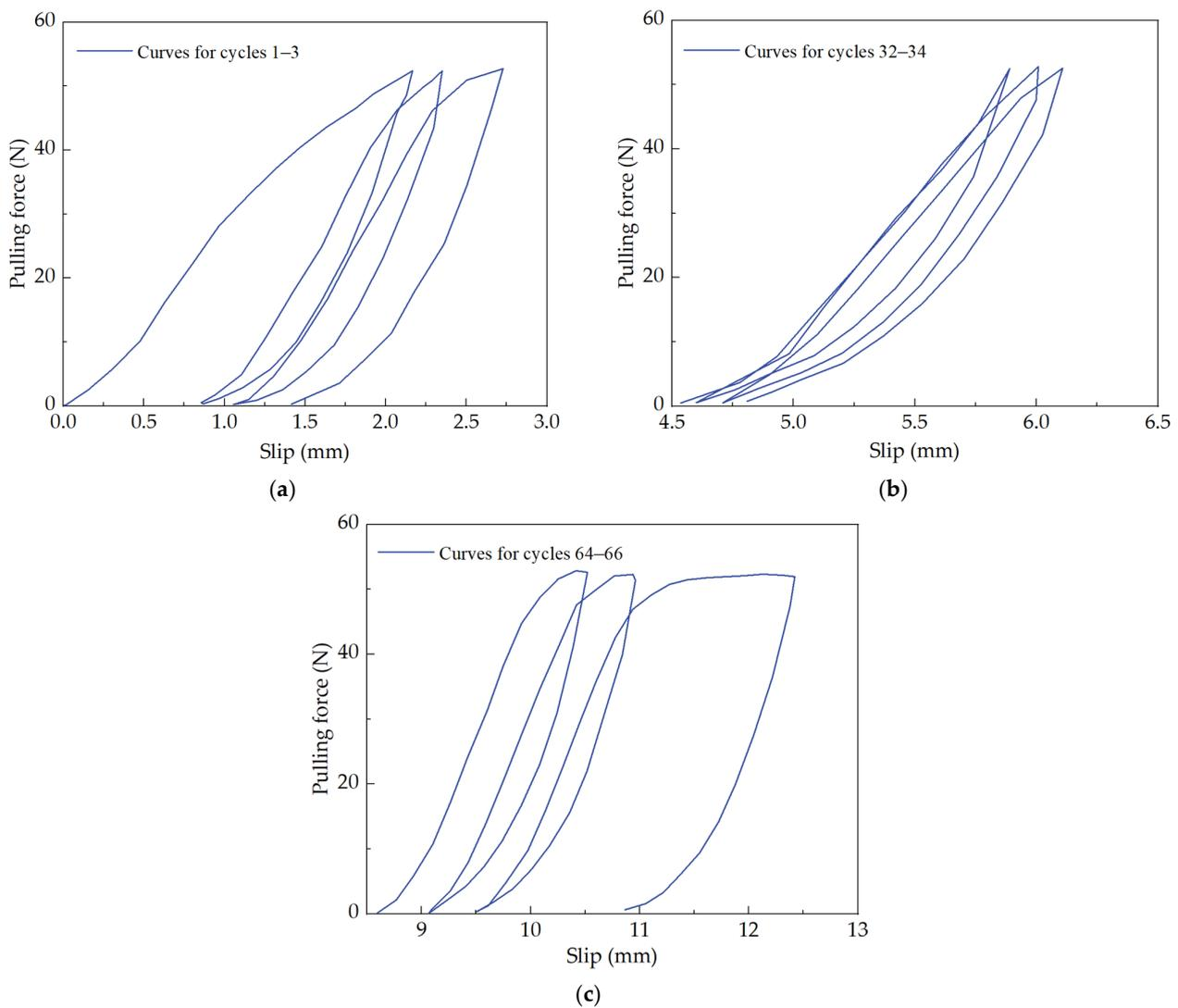
**Figure 9.** Evolution of pull-out force–slip hysteretic curve under 75% cyclic loading amplitude. (a) Loading and unloading section of the 1st–3rd cycle. (b) Loading and unloading section of the 32nd–34th cycle. (c) Loading and unloading section of the 64th–66th cycle.
