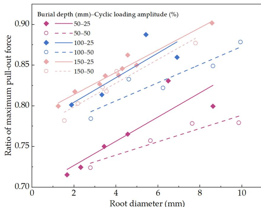
**Figure 13.** Influence of burial depth and cyclic loading amplitude on the ratio of maximum root pull-out force before and after cyclic loading.
