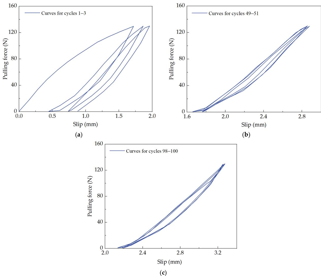
**Figure 8.** Evolution of pull-out force–slip hysteretic curve under 50% cyclic loading amplitude. (a) Loading and unloading section of the 1st–3rd cycle. (b) Loading and unloading section of the 49th–51st cycle. (c) Loading and unloading section of the 98th–100th cycle.
