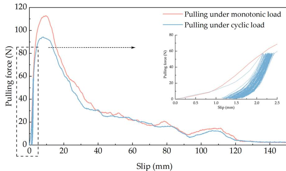
**Figure 4.** Pull-out force–slip curve of failure mode 1 and comparison of curves under different loading modes.
