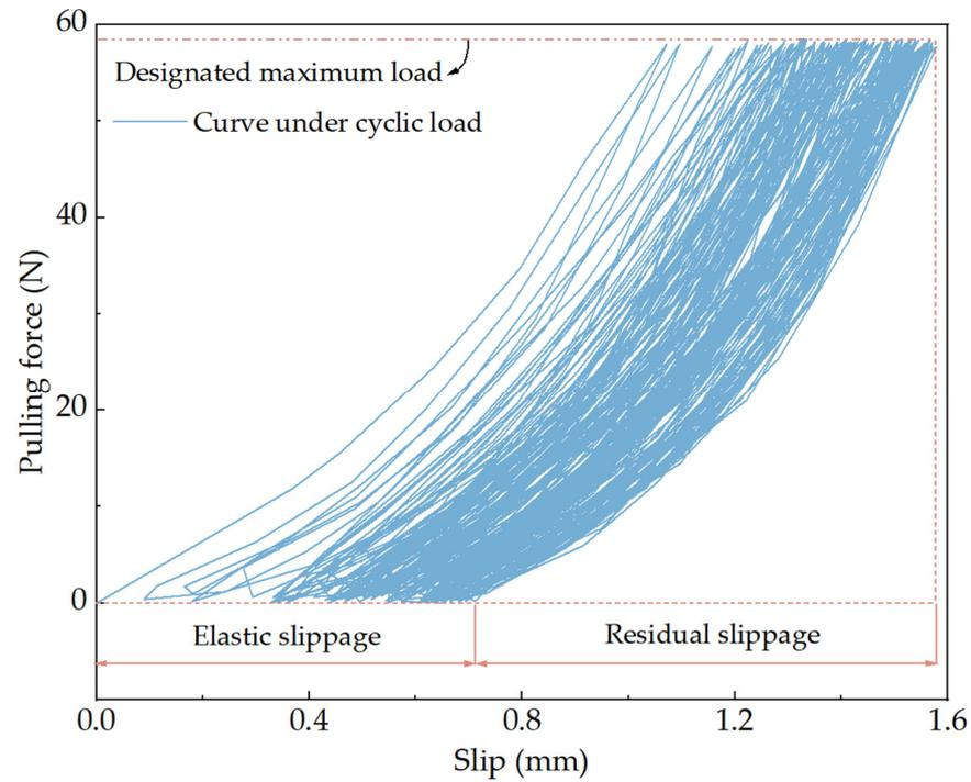
Figure 6. Pull-out force–slip cycle segment curve.
