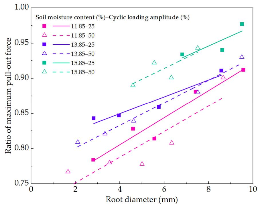
**Figure 12.** Influence of soil moisture content and cyclic loading amplitude on the ratio of maximum root pull-out force before and after cyclic loading.
