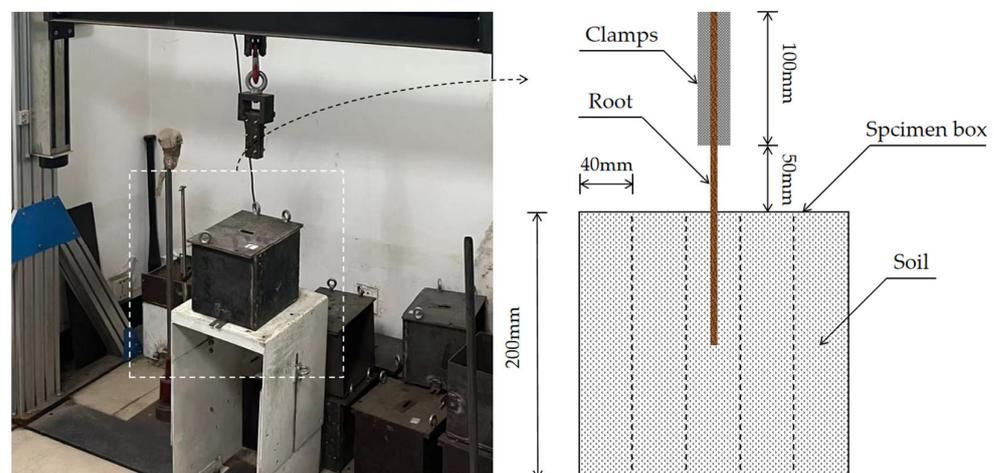
**Figure 3.** Test machine and specimen system.
