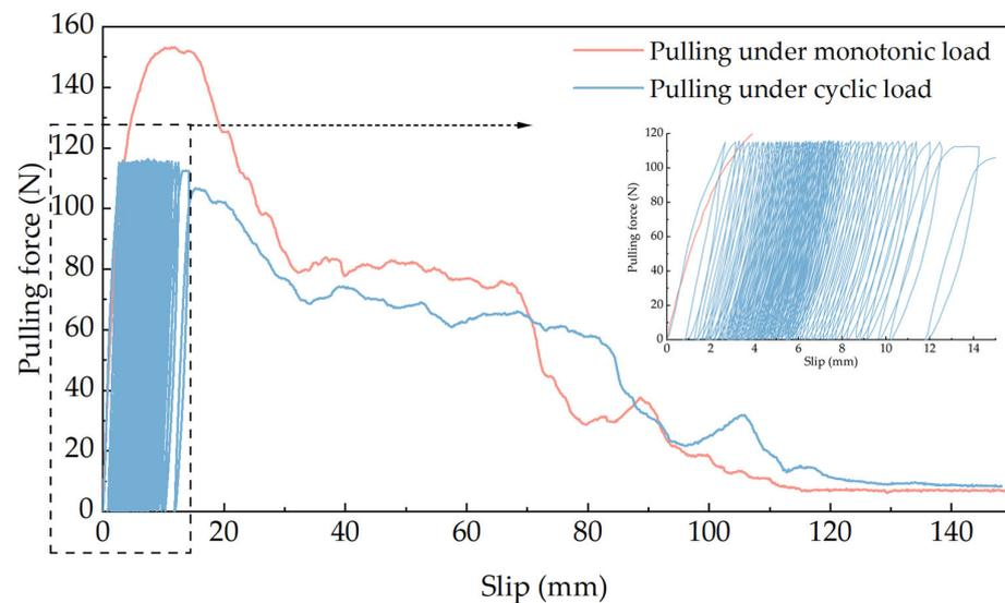
**Figure 5.** Pull-out force–slip curve of failure mode 2 and comparison of curves under different loading modes.
