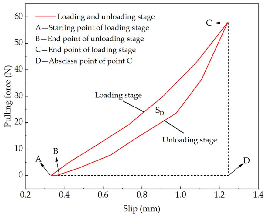
Figure 7. Characteristic cycle loading and unloading section.
