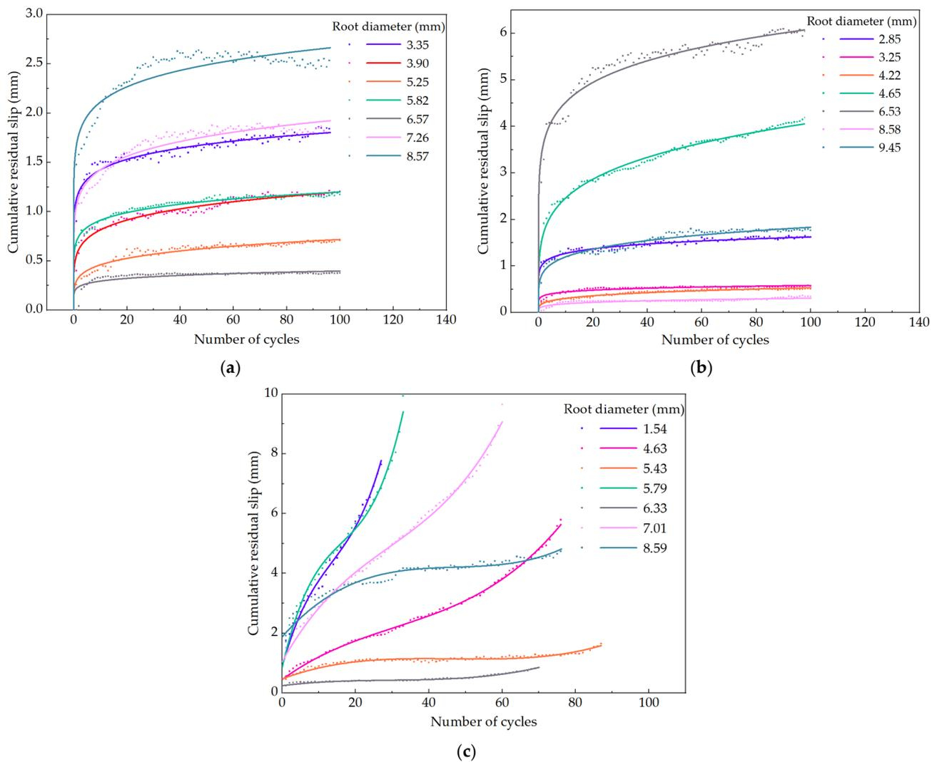
**Figure 10.** Trend of cumulative residual slip. (a) At 25% cyclic loading amplitude. (b) At 50% cyclic loading amplitude. (c) At 75% cyclic loading amplitude.
