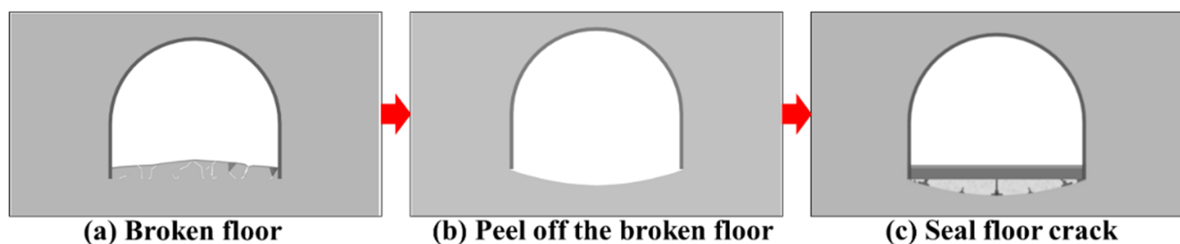
Figure 14. Inverted arch in the roadway.
